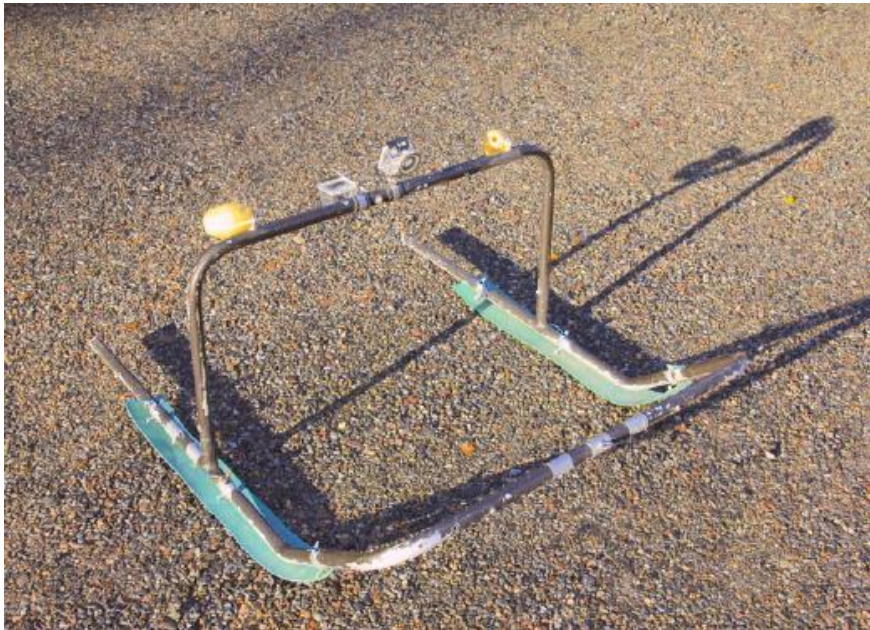
Figure 7. The equipment for benthic litter monitoring by towed camera developed by Lundquist 123
