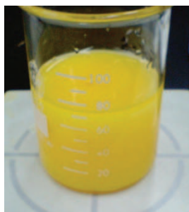
Figure 6 The \text{Cs}_2\text{Pt}(\text{Cl})_4 precipitate at step 18
