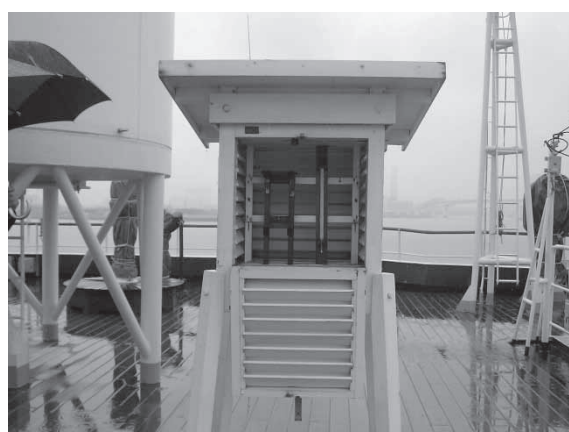
Fig. 3.5 Instrument shelter called "Screen" in which a psychrometer is housed
