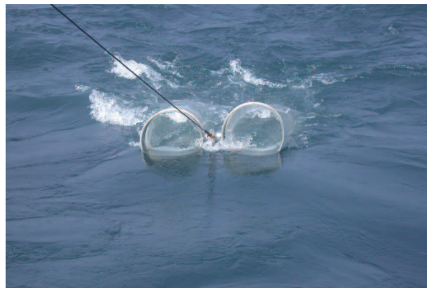
Fig. 3 BONGO net (70 cm ring diameter). Photo by Dr. Y. Okazaki.
