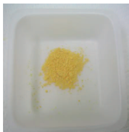
Figure 7 Dry upped Cs_2Pt(Cl)_4 precipitate at step 20
