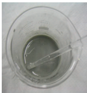
Figure 4 Dissolve AMP/Cs compound by adding alkali solution at step 14
