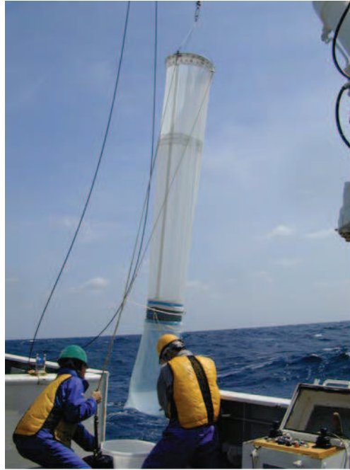
Fig. 2. A plankton net attached large plastic bag as a cod end to collect living zooplankton for incubation experiment.
