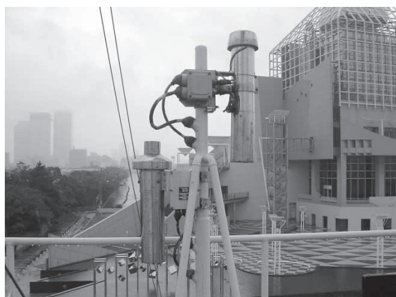
Fig. 3.4 Electric thermometer and hygrometer housed in separate metal envelopes
