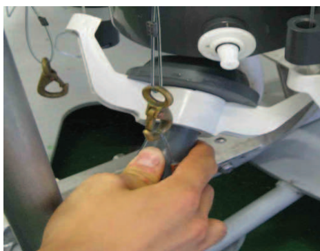
Photo A.1-2-1 Checking tension of lower lid lanyard. Photo A.1-2-2. Checking tension of upper lid lanyard.
