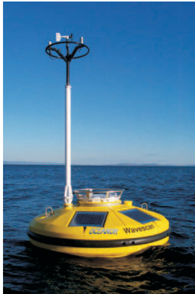
Figure 4.1: The Wavescan heave/pitch/roll data buoy, \text{Ø}2.8\text{ m} (Photograph used by permission).
