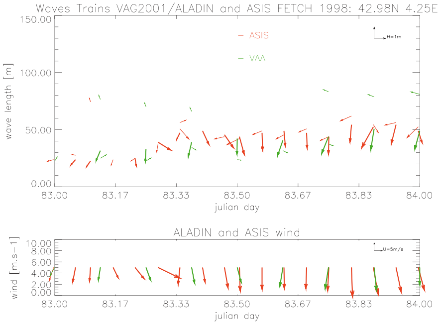
Figure 10.2: Mean direction (arrows direction), wavelength corresponding to the mean period (y axis) and height (proportional to the length of the arrows) of the wind sea and the total swell on March 24 th 1998 as a function of time (horizontal axis). Green vectors are for the model. Red vectors are for the ASIS buoy data.
