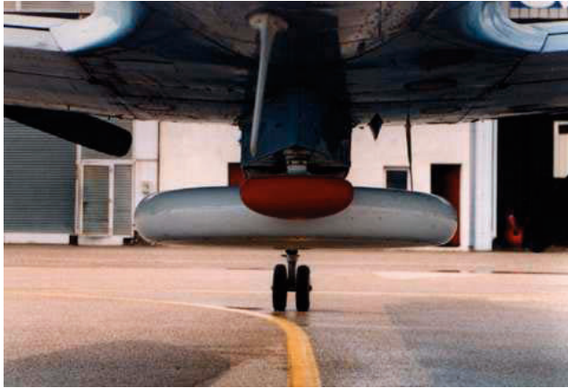
Figure 5.18: View of the antenna of RESSAC mounted below the fuselage of the MERLIN-IV. The small radome contains the transmitting antenna, The large one the receiving antenna. Both rotate around the vertical axis at a speed of 1 rotation per minute.
