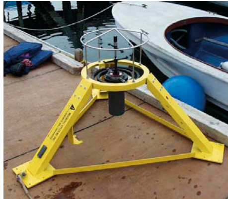
Figure 4.7: The 3D-WAVE Acoustic Current Meter manufactured by Falmouth Scientific ( Photograph used by permission ).
