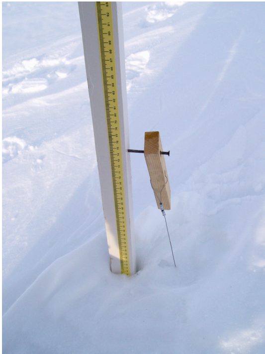
Above left: A hotwire gauge with handle hanging on nail above the snow. Photo: Teema Qillaq. Above right: Toku Oshima and Teema Qillaq pull up on a heated hotwire cable and measure the length of the cable, as described in Section 3.3. Photo: Andy Mahoney
