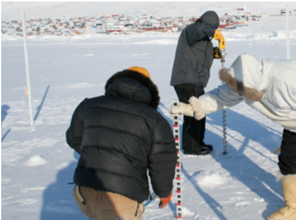
Placing snow stakes for a monitoring station near their community of Qaanaaq, Greenland, Andy Mahoney and Mamarut Kristiansen insert a snow stake into a hole in the ice, taking care to ensure it is vertical. In the background, Joe Leavitt drills a hole for another stake. Photo: Shari Gearheard
