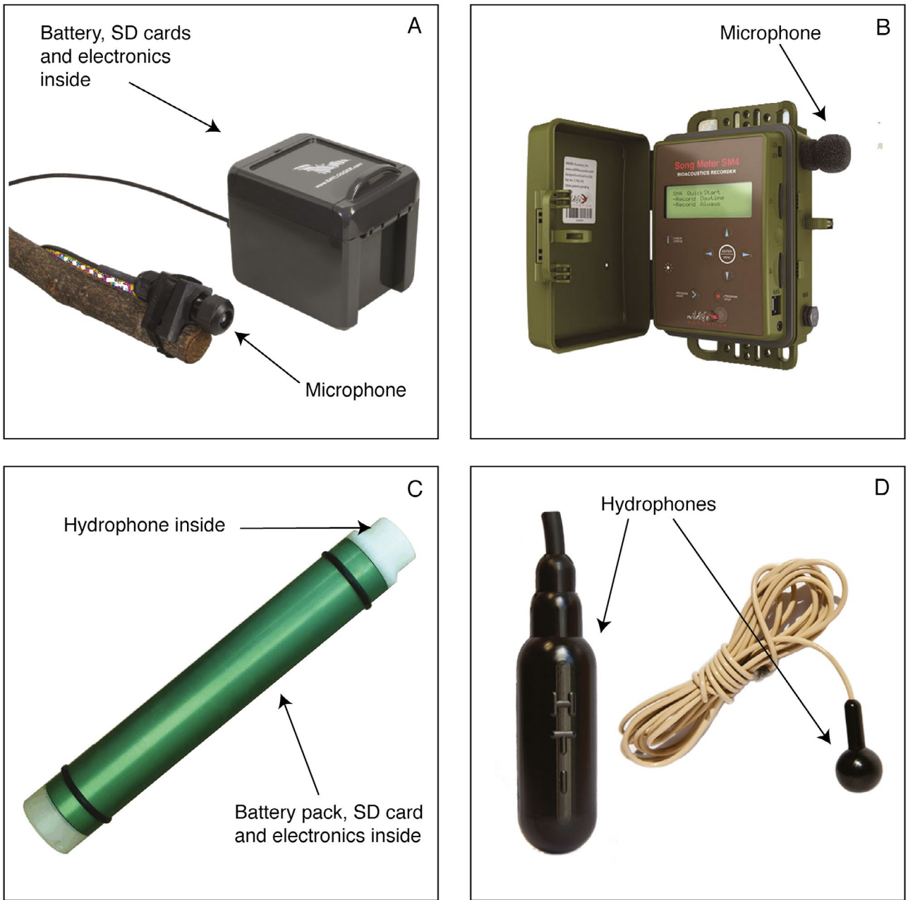
Figure 4: A selection of commercially available bioacoustic sensors, shown for illustrative purposes. These include audible range and ultrasonic sensors for both terrestrial (A: Elekon Batlogger and B: Wildlife Acoustics SM4) and aquatic environments (C: Chelonia Ltd. Deep C-POD and D: High Tech Inc. HTI-99-HF hydrophones).
