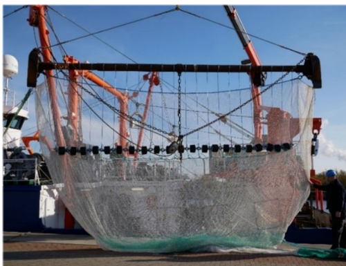
Figure 5: Left: Straight ground gear (left) and comparison of regular ground gear with axial-offset roller ground gear (von-Holdt type, right).
