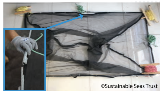
Figure 7.6: To assemble the STOP net, open the net, place it squarely on the ground, and click the frame together. Note that there is an anti-twist section on one side of the frame to prevent the frame from twisting.
