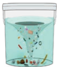
Figure 4.8: Meso-litter particles floating in a bucket of swirled seawater. The floating meso-litter particles can easily be collected, while items such as seashells sink to the bottom of the bucket faster than the plastic particles.
