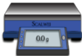
Figure 3.12: Litter should be weighed per type of litter to the nearest 0.1 g.
