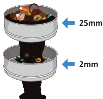
Figure 7.15: After removing all visible non-litter items, sieve the remaining material through stacked sieves with 25 mm and 2 mm mesh
