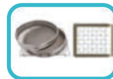
9. Stackable test sieves OR 50 x 50 cm framed sieves with mesh sizes of 2 mm & 25 mm
