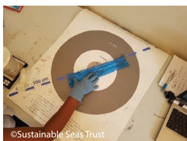
Figure 7.17: Appendix 4 can be used to sort macro-litter fragments into different size classes as required.
