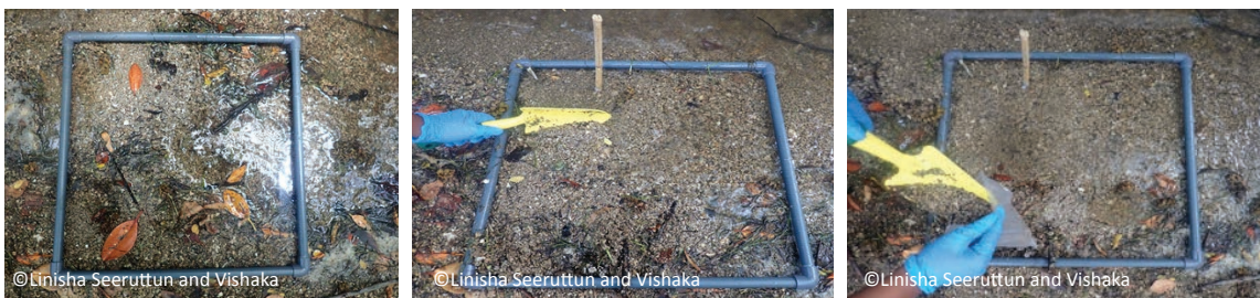
Figure 6.3. Sample collection for meso-litter using 50 x 50 cm quadrats. A small measured stick is used as a ruler to indicate depth.
