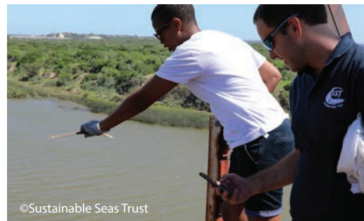
Figure 7.4: River flow rate can be measured using the stick/orange peel methods.
