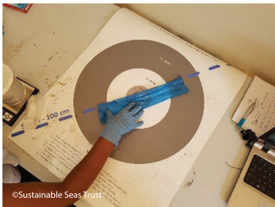
Figure 8.8: Appendix 4 can be used to sort litter fragments into different size classes as required.
