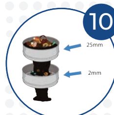
10 WASH REMAINING SEDIMENT OVER SIEVES
