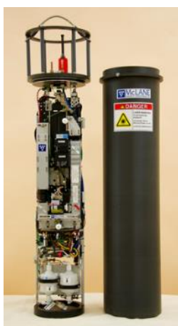
Figure 3.1.1 The imaging FlowCytobot with the pressure proof housing removed.
