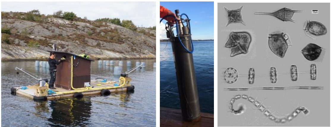
Figure 3.1.12. An automated underwater microscope, the Imaging FlowCytobot was used next to a mussel farm in Sweden August to October 2016. An automated winch was used to move the instrument to different depths. The collage of images to the right shows images collected using the IFCB illustrating some of the phytoplankton observed.
