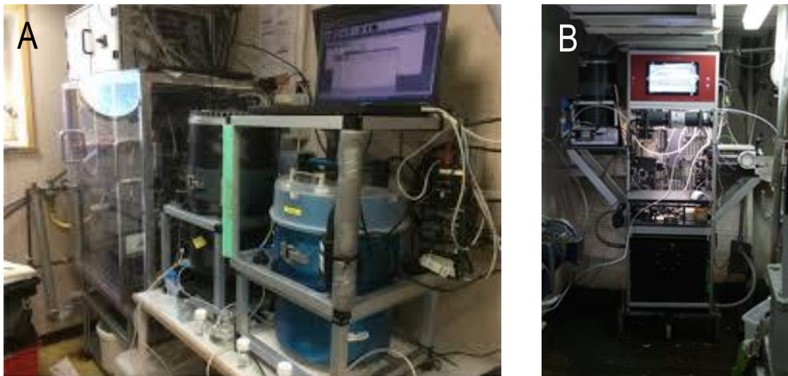
Figure 3.2.10. 2 CytoSenses side by side connected onboard the RV CEFAS Endeavour (A) and onboard the "Le Carthage". They are connected to the 4H-JENA FerryBox.
