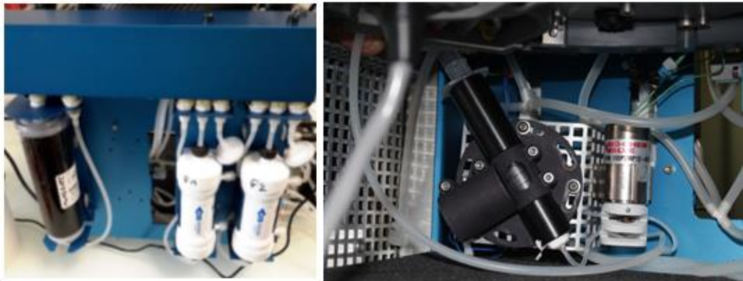
Figure 3.2.12. Beads-Sheath-Toxins (BST) system with coal filter and classical 0.1 µm filter ensure long life clean sheath fluid.
