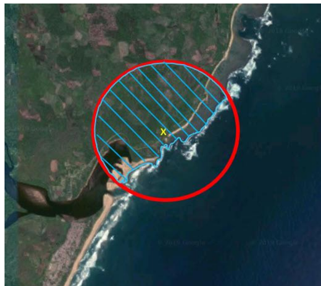
Figure 15. Example of using spatial fit on the results of both a point-radius method and a refined shape method of describing uncertainty. Assuming the blue-shaded area is the "true" locality as we know the species is terrestrial, and the red circle is the point-radius method of representing the uncertainty, the ratio of the area of the red circle (5.726 sq km) divided by the area of the blue shaded area (~4.1 sq km) gives a spatial fit for the point-radius of 1.39.
