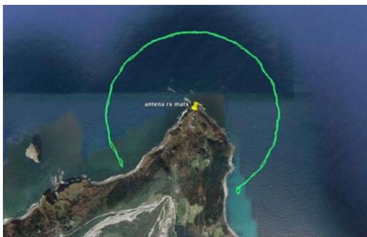
Figure 1 – Trajectory (in green) of the boat carrying the transponder used to calibrate the antenna of Matxitxako (Basque County HFR network in the SE Bay of Biscay) in September 2014. Yellow marker shows the position of the receiving antenna (courtesy of QUALITAS).
