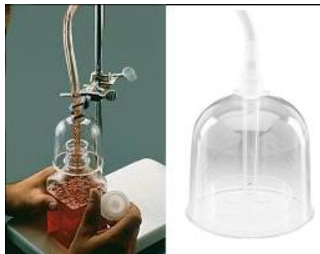
Figure A2. Polycarbonate filling bell (Nalgene, Thermo Fisher Scientific Inc., part number DS03900070).
