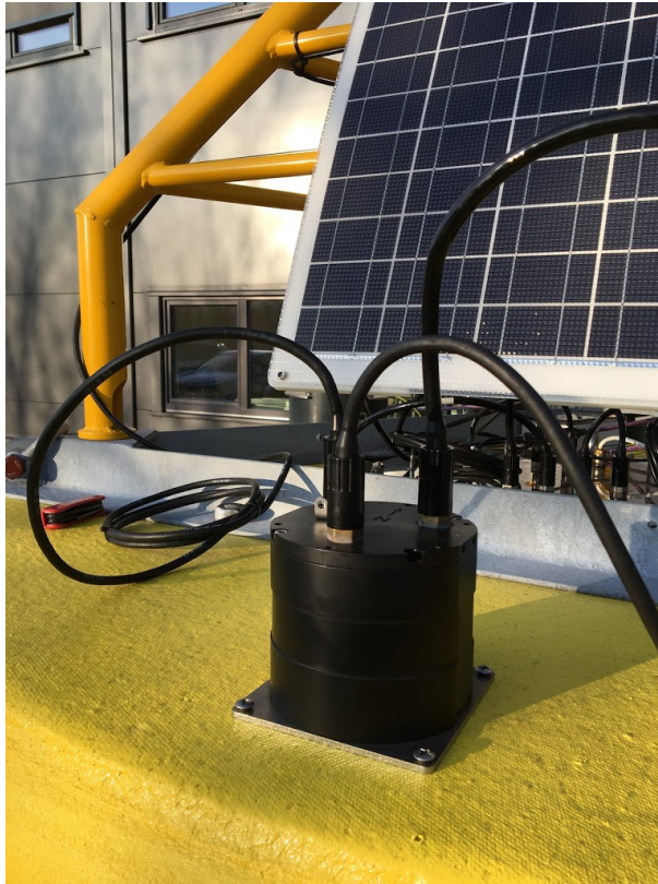
Figure 10-4: Sensor mounted with horizontal mounting plate
