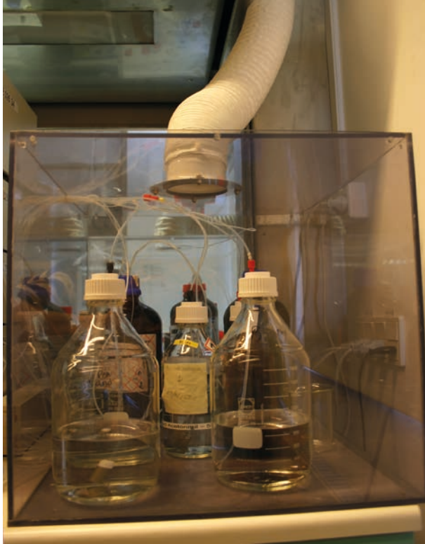
Ventilated storage of hazardous chemicals is essential (Elmer Topp-Jørgensen/Aarhus University).
