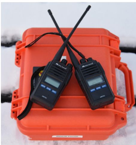
Figure 3.7 Small handheld VHF radios are ideal for short distance communication between field teams. Photo: Morten Rasch.
