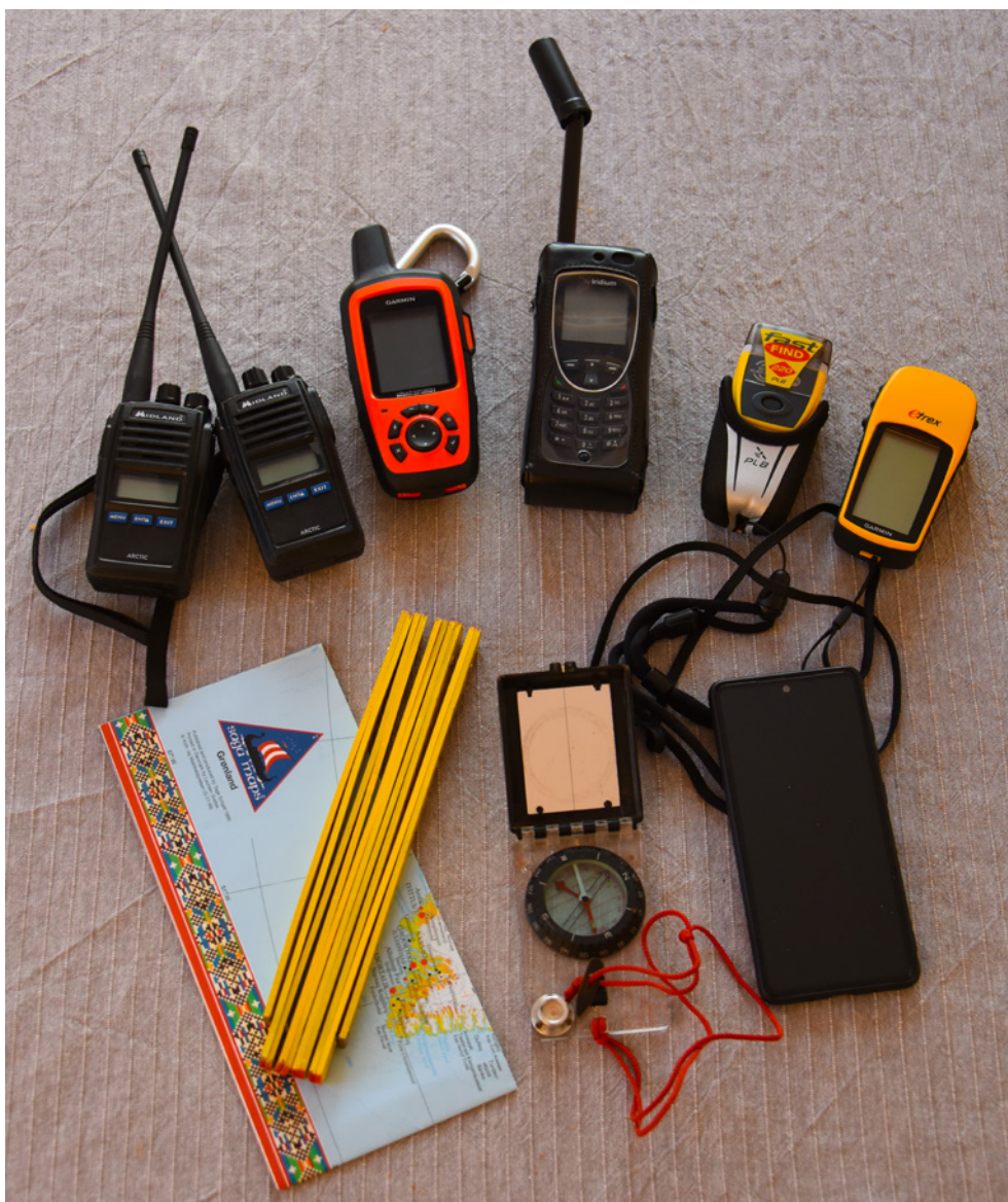
Figure 1.1 Different devices for communication and navigation. Upper row from left to right: VHF radios, InReach, Iridium phone, Personal Locator Beacon and GPS. Lower row: Map and ruler, compass and mobile phone. Photo: Morten Rasch.
