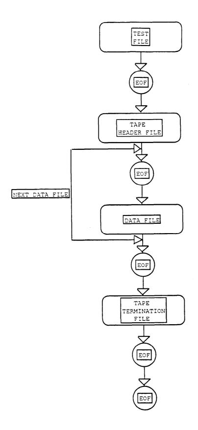
FIGURE 1. GF-3 TAPE STRUCTURE
