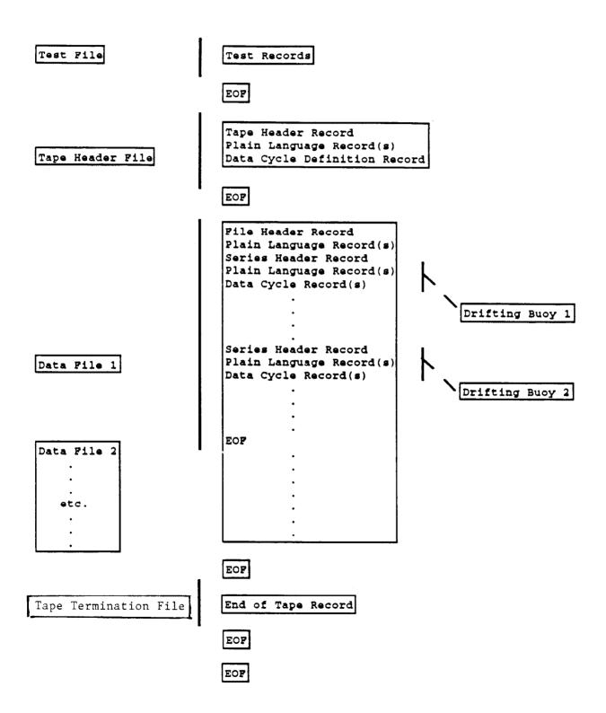
FIGURE 9. STRUCTURE OF A GF-3 TAPE FOR DRIFTING BUOY STANDARD SUBSET
