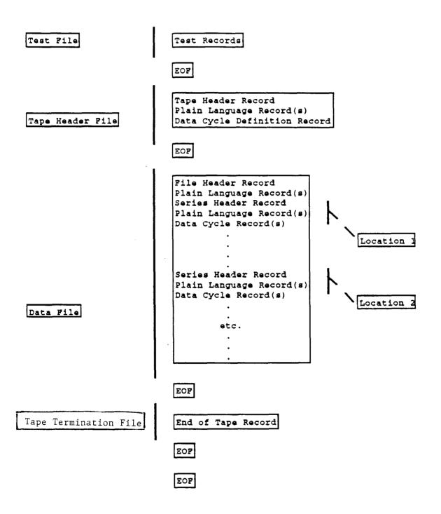
FIGURE 7. STRUCTURE OF A GF-3 TAPE FOR MEASURED WAVE SPECTRA SUBSET
