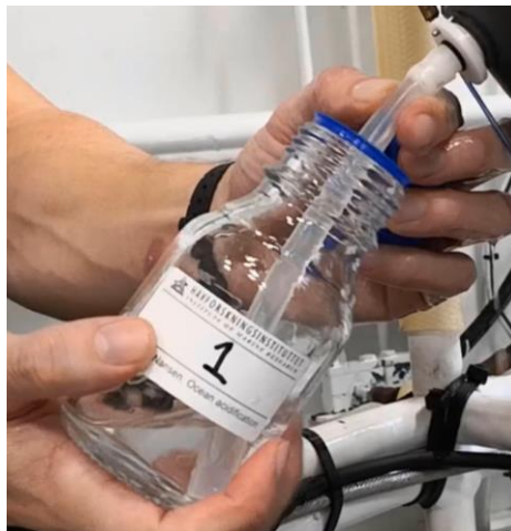
Figure 3. Sample bottle for a pH/total alkalinity sample being filled. Notice that the silicone tube is at the bottom of the bottle and the tube is in the process of being pinched (repeatedly).
