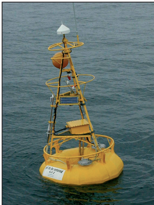
Figure 8.3 The GFZ Potsdam GPS buoy.
