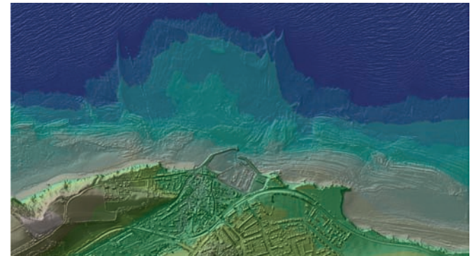
Fig. 4.1. LIDAR digital surface model for coastal terrain and nearshore seabed mapping This example, showing bathymetric zonation and seabed morphology, is from Watchet in England, United Kingdom
