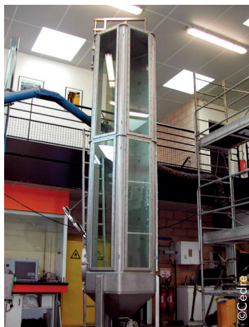
Experimentation column to study the behaviour of a chemical (or oil) as it rises or sinks in the water column.
