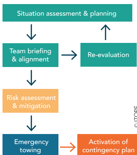
Figure 67: Suggested steps in emergency tow planning
