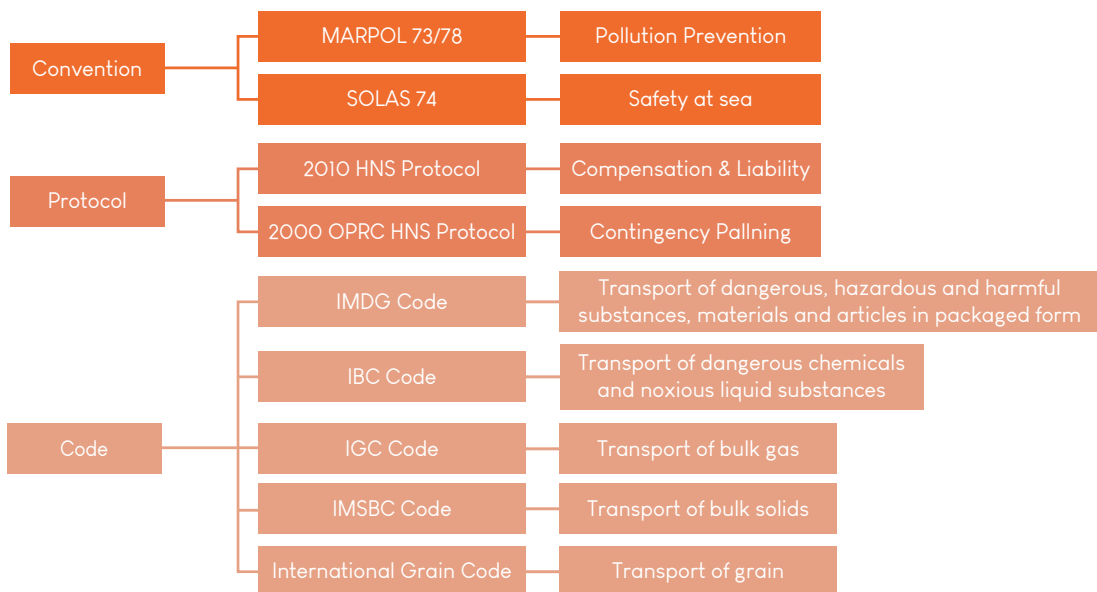
Figure 2: IMO conventions, protocols and codes relevant for the transport of HNS at sea
