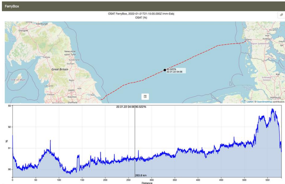
Figure 7-12: SOS V2 plot of the transect Immingham-Esbjerg (22.01.2022). Shown are the measured data for oxygen saturation in a spatial as well as temporal representation
