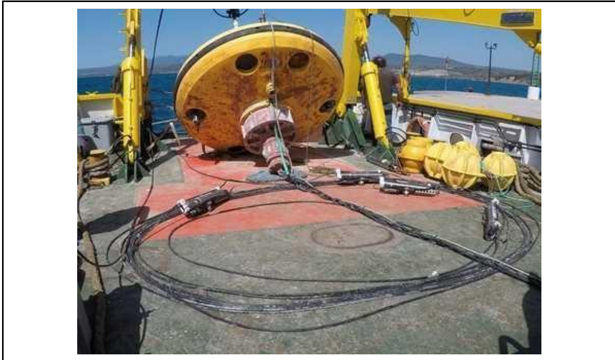
Figure 5-7: The buoy with the first 100 metres of inductive cable arranged at the stern of the ship before deployment.
