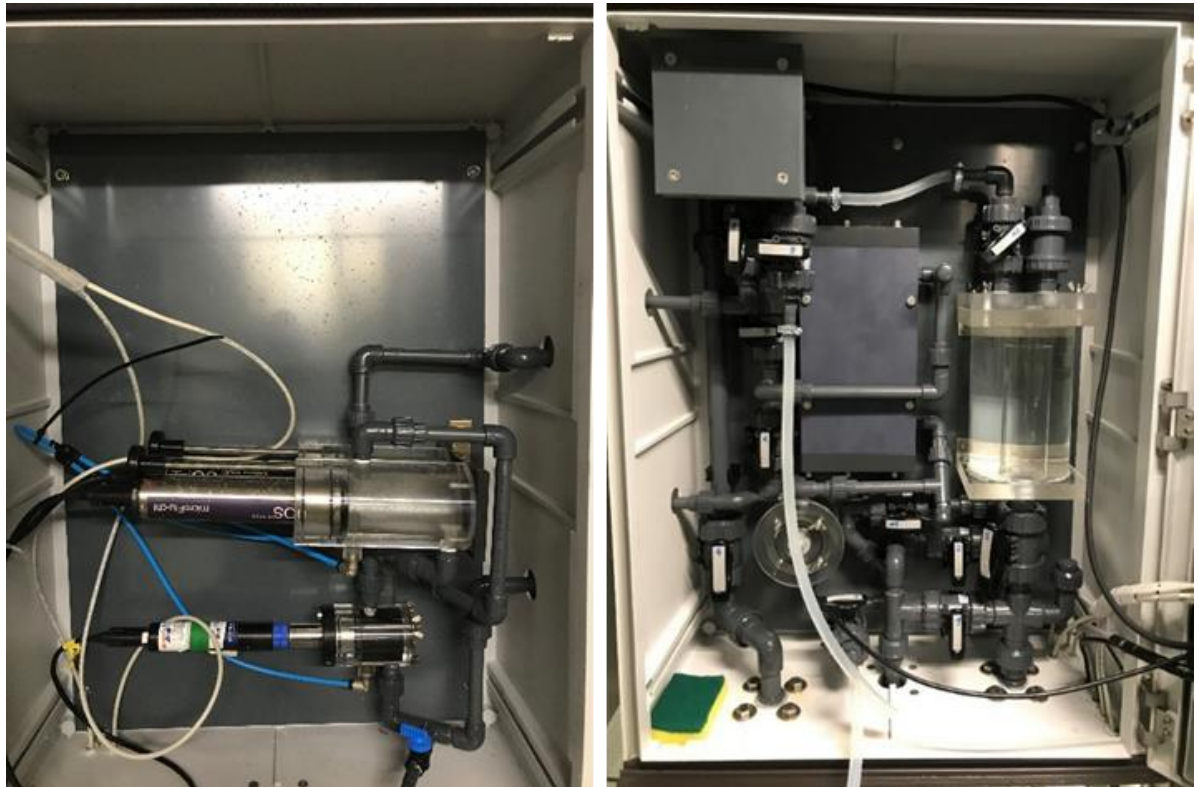
Figure 7-2: NIVA FerryBox. Left panel - optical/fluorescence sensors and flow cells; right panel - clear cylinder = debubbler, gray rectangle in center = SBE45 CTD, clear circle below SBE45 = oxygen optode:
