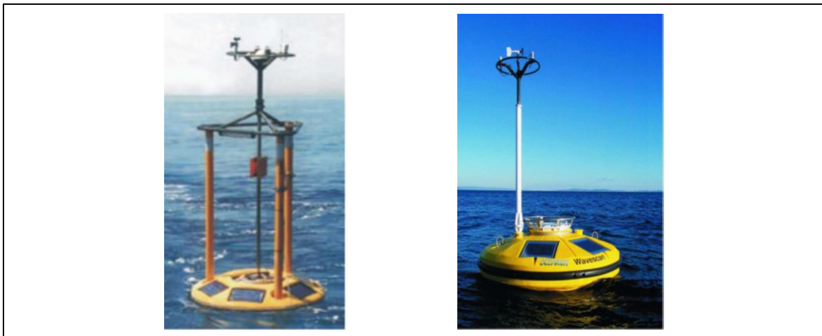
Figure 5-4: Picture of the SEAWATCH and wavescan type of buoy, respectively
