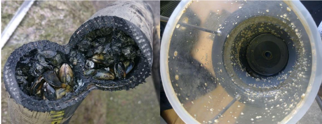
Figure 7-3: Examples of biofouling in intake tubing (left image : mussels, barnacles) and debubbler (right image : barnacles growth 2 weeks after cleaning) at Cuxhaven Stationary FerryBox, located at the mouth of Elbe Estuary. Image courtesy of Hereon (H. Rust, M. Gehrung).
