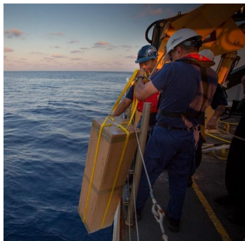
Figure 5: Deployment of the Argo float within a box over the side of the vessel (Photo: WHOI)
