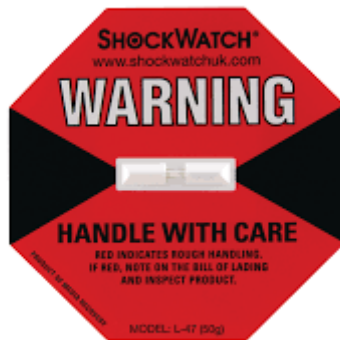
Figure 4: Shock absorber glass tube. If the tube is red, the Argo float was not handled correctly.
