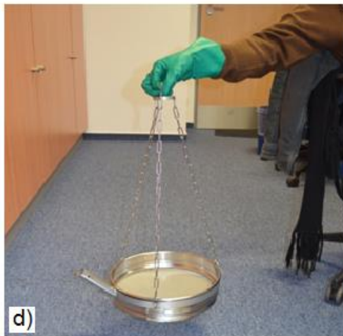
Figure 1: Screen sampling devices. a) Drawing of a typical screen sampler; b) Rectangular screen sampler equipped with a handle for working close to the water surface; c) Rectangular screen sampler in a protective cover for transportation; d) Round screen sampler, factory-welded into a frame (Linker Industrietechnik No. 553055222056, originally manufactured for grain size classification, according to ASTM MESH 16), with lid, bottom and three-point chain suspension. The sampler is operated by rope; e) Round screen sampler and transportation covers.
