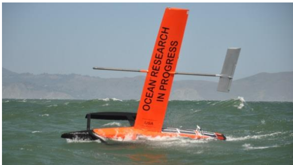
Figure 13: Picture of Sairdrone. Length: 19 ft. Width: 7 ft. Height: 20 ft above water surface. Draft: 6 ft below water surface. Average speed: 3-5 knots. Maximum speed: 14 knots. Payload power available: 5-10 W. Deployment duration: 6-8 Months.
