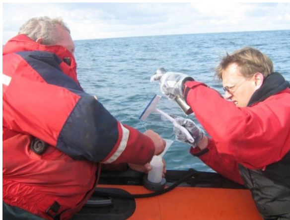
Figure 1: Sampling with a glass plate from a Zodiac boat.
