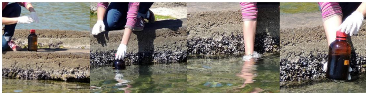
Figure 2: Sampling of the bulk subsurface water by “hand-dipping” for samples.
