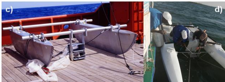
FIGURE 19. General view of the five-stage plankton-neuston net (Zaitsev, 1964a)
