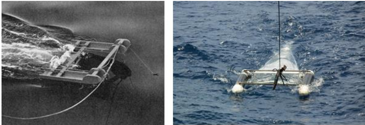
Figure 4: Neuston net mounted in front of the floating elements (picture a) adapted from Bieri and Newbury, 1966; picture b) by Miguel Leal).
