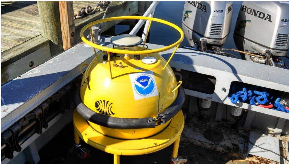
Figure 2-7. This AXYS GPS water level buoy is ready to be deployed by NOAA/NOS for evaluation in the southern Chesapeake Bay (courtesy of Mark Bushnell, CoastalObsTechServices).
