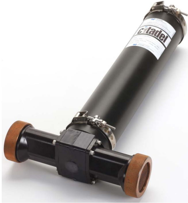
Figure 2-5. The TRDI CITADEL CTD-NH is an example of an inductive sensor with a constrained field (photo courtesy of Paul Devine/TRDI).
