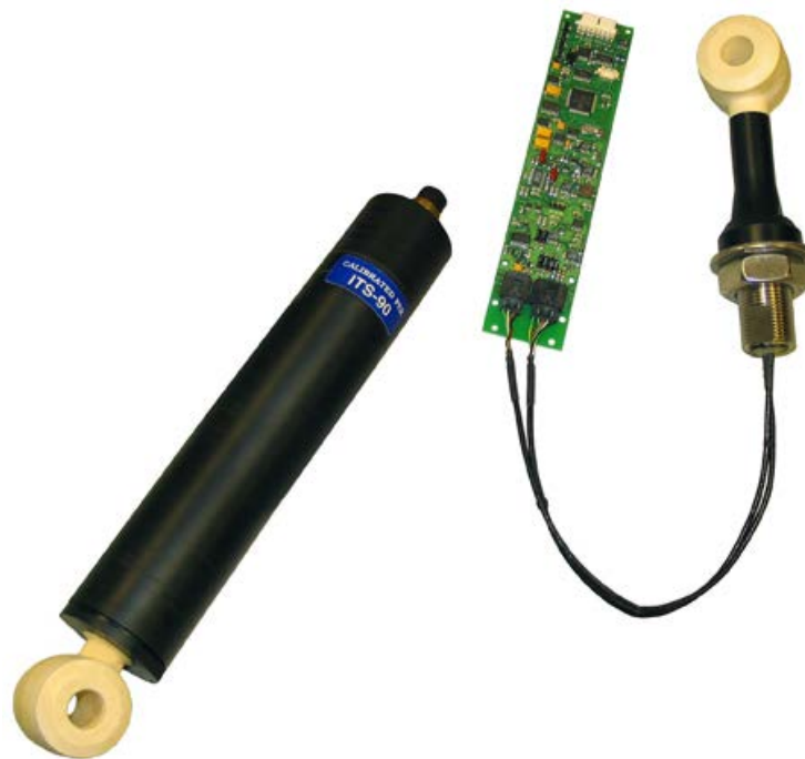
Figure 2-4. The TRDI CITADEL CTD-ES is an example of an inductive sensor with an external field. Operators must be certain that additional hardware is sufficiently distant from the toroid to avoid interference. This sensor is designed for simple and easy cleaning (photo courtesy of Paul Devine/TRDI).
