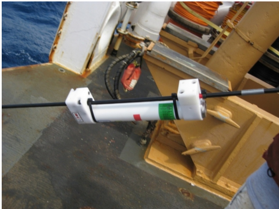
Figure 2-2. This Sea-Bird SBE-39-IM temperature and pressure recorder uses an inductive modem to transmit data up the mooring cable to a surface receiver (photo courtesy of Karen Grissom/NOAA NDBC).
