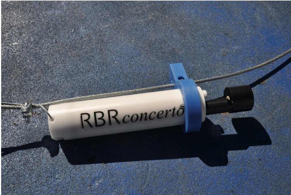
Figure 2-3. This towed RBR concerto CTD uses an inductive sensor with an external field and no pump (photo courtesy of Igor Shkvorets/RBR).
