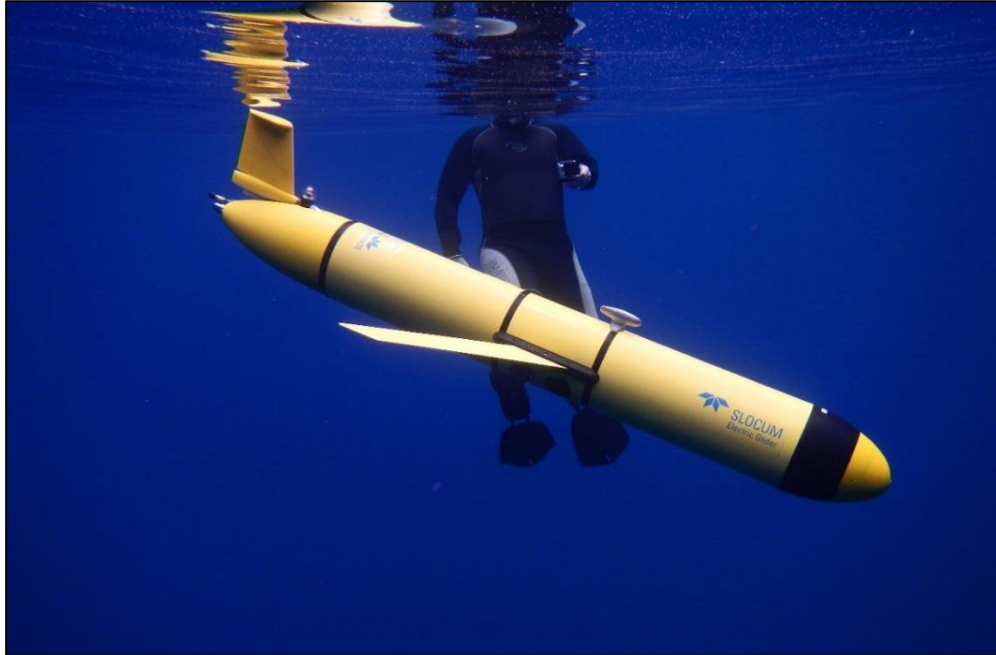
Figure 1. Slocum glider (photo courtesy of Rutgers University).
