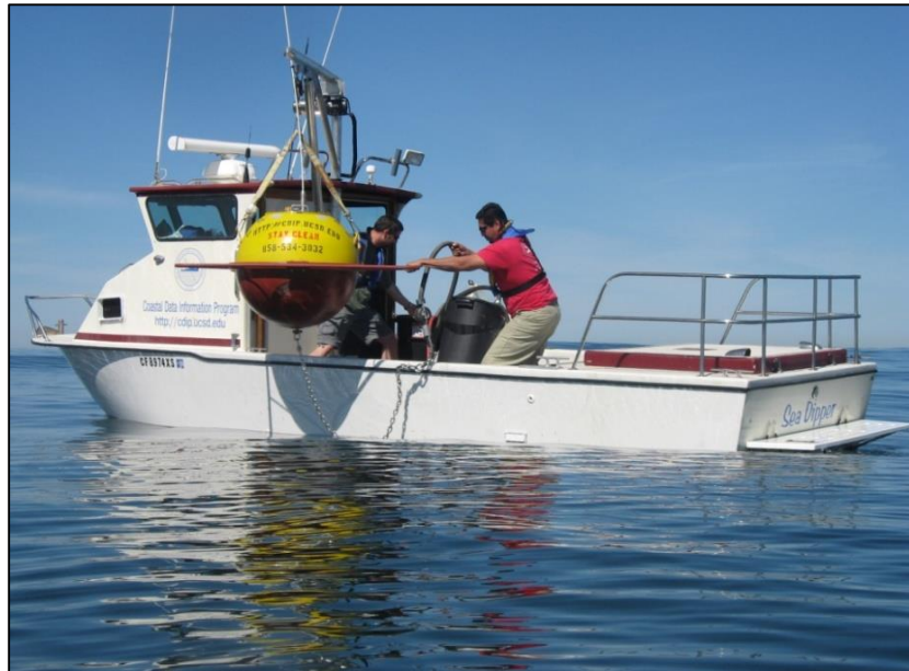
Figure 2-3. CDIP personnel deploy a Datowell directional Waverider. As of 2015, the CDIP network is composed of approximately 60 wave observation sites. (Photo courtesy of SIO/CDIP)
