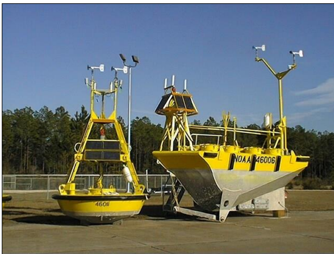
Figure 2-1. NDBC 3-m discus buoy (left); NDBC 6-m NOMAD buoy (right). (Photo courtesy of Richard Bouchard/NDBC)
