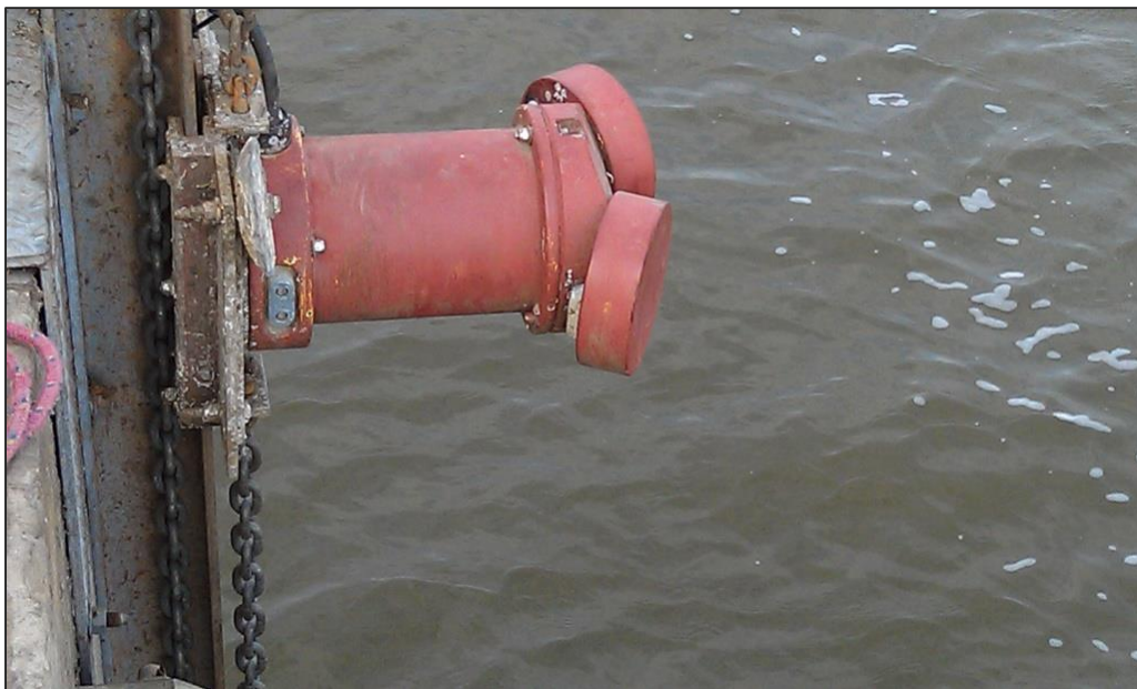
Figure 3-5. A SonTek side-looking ADP is raised for cleaning. (Photo courtesy of Warren Krug/NOAA)
