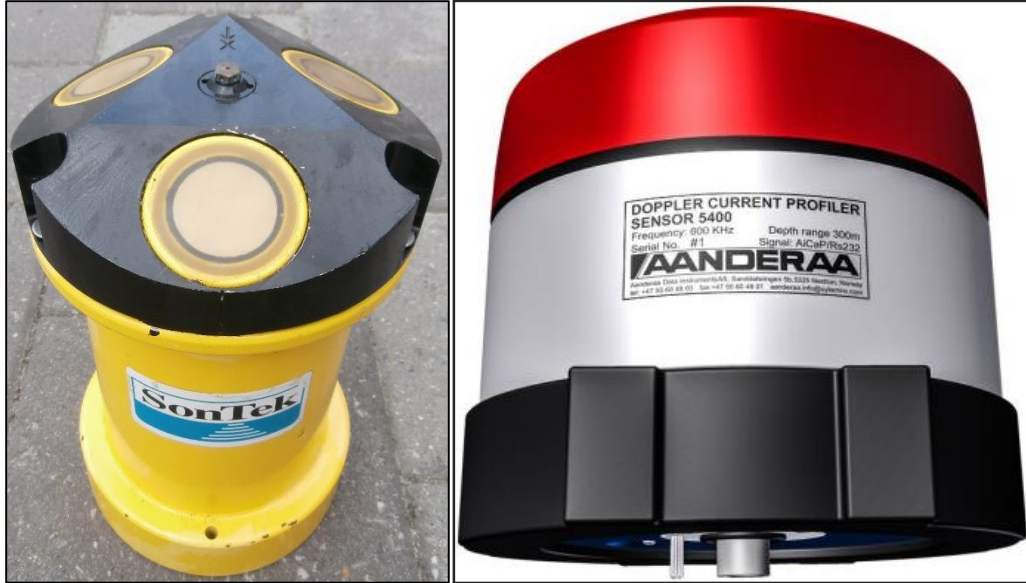
Figure 3-2. SonTek ADP (left); Aanderaa Doppler current sensors (right). (Photos courtesy of Mark Bushnell/NOAA and Aanderaa website)
