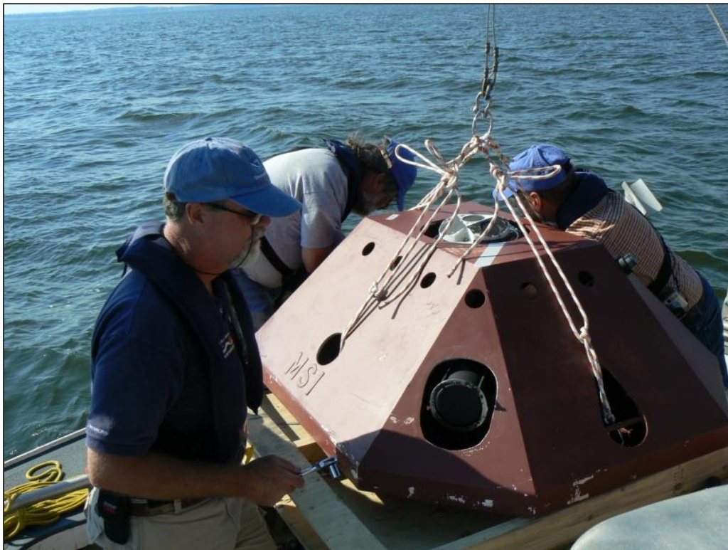
Figure 3-4. A bottom-mounted upward-looking Nortek AWAC is prepared for deployment. (Photo courtesy of Doug Wilson/NOAA)
