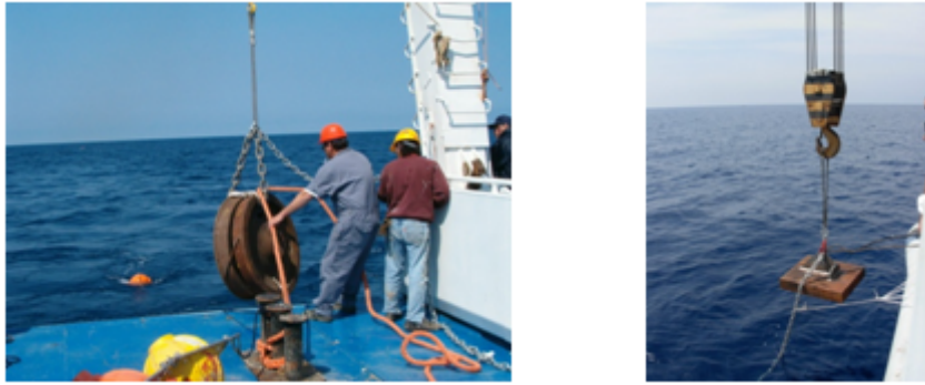
Figure 1.2.1 a Deployment of mooring anchor
