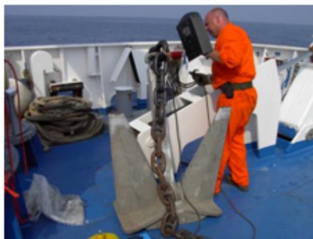
Figure 1.2.2 b: Typical anchor used for buoy deployment
