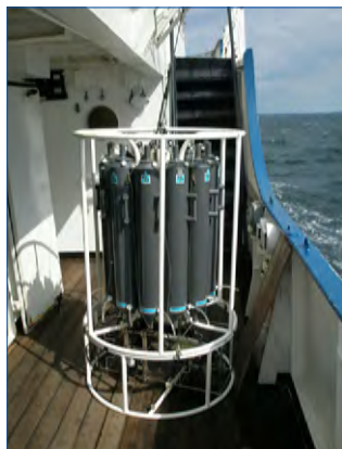
Figure 4. CTD with rosette and Niskin-type water bottles. An in situ chlorophyll a fluorometer is also mounted.
