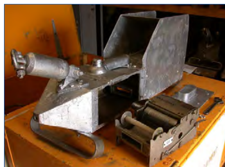
Figure 7. The Continuous Plankton Recorder. This device is mainly aimed for sampling zooplankton but may be useful for collecting larger, non fragile phytoplankton species. Photo courtesy of the Sir Alister Hardy Foundation for Ocean Science, SAHFOS http://www.sahfos.ac.uk/ .
