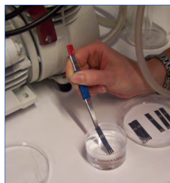
Figure 10. Washing of chips in a petri dish with wash buffer.
