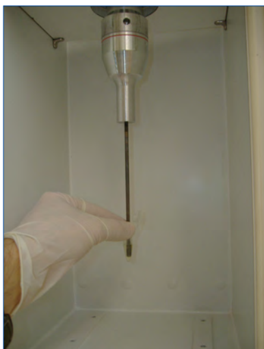
Figure 5. Cell lysis by sonication.
