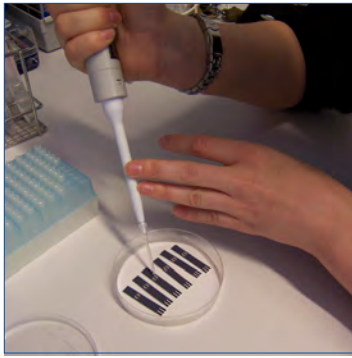
Figure 6: Applying of buffer onto the electrodes.
