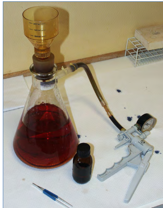
Figure 1. Filtration manifold and hand held vacuum pump.
