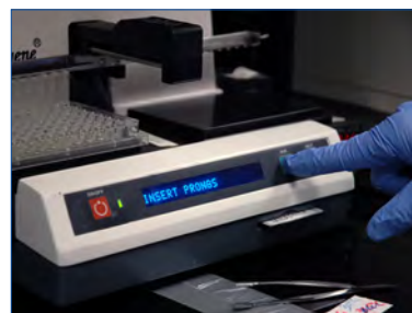
Figure 9. Processor being started after plate is positioned on heater base.
