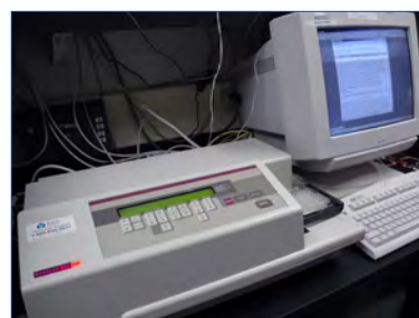
Figure 10. Microplate is placed on microplate reader cradle; optical density is recorded at 650nm for row "A" (wells in which colour development has occurred).
