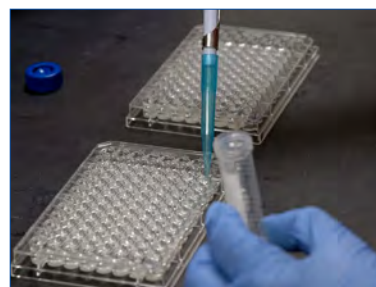
Figure 7. Lysate (0.25 mL) is added to appropriate sample wells on microplate.
