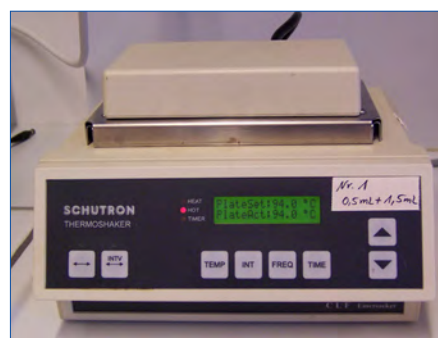
Figure 11. Schutrone ThermoShaker for the fragmentation and denaturation of the sample.
