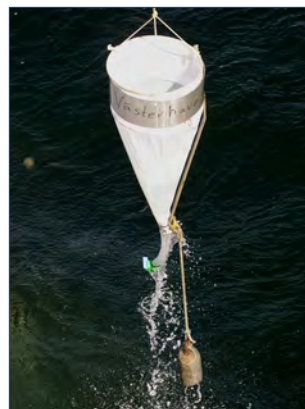
Figure 5. Phytoplankton net. This is not used for quantitative sampling but for collecting rare, non fragile species.
