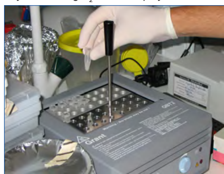
Figure 6. Samples in a thermal block at 55 °C.
