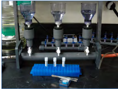
Figure 3. Three-position vacuum filter manifold used to collect particulate fraction of water sample.
