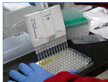
Figure 11. After microplate is read at 650nm, row "A" is acidified with 50 µL of 10% H 2 SO 4 ; optical density is recorded at 450 nm for row "A". The measure at 650 nm is considered low sensitivity while that at 450 nm is considered high sensitivity. For positive samples, the optical density at 450 nm should be roughly 2X that at 650 nm.
