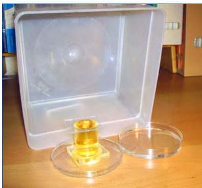
Figure 8. Sedimentation, with a Petri dish filled with water. A plastic box covers the sedimentation chamber and the Petri dish to maintain the humidity.
