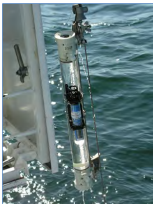
Figure 2. Reversing water sampler of the modified Nansen type.
