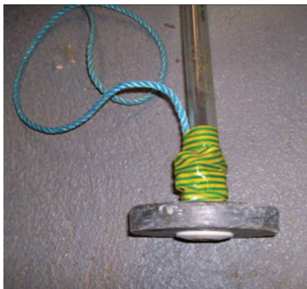
Figure 5. Lund's tube sampler with disk-shaped plumb bob that encircles the bottom end of the tube.
