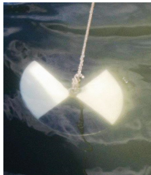
Figure 2. Various models and parts of a Secchi disk; view of a disk submerged in water with plenty of greenish pigments.
