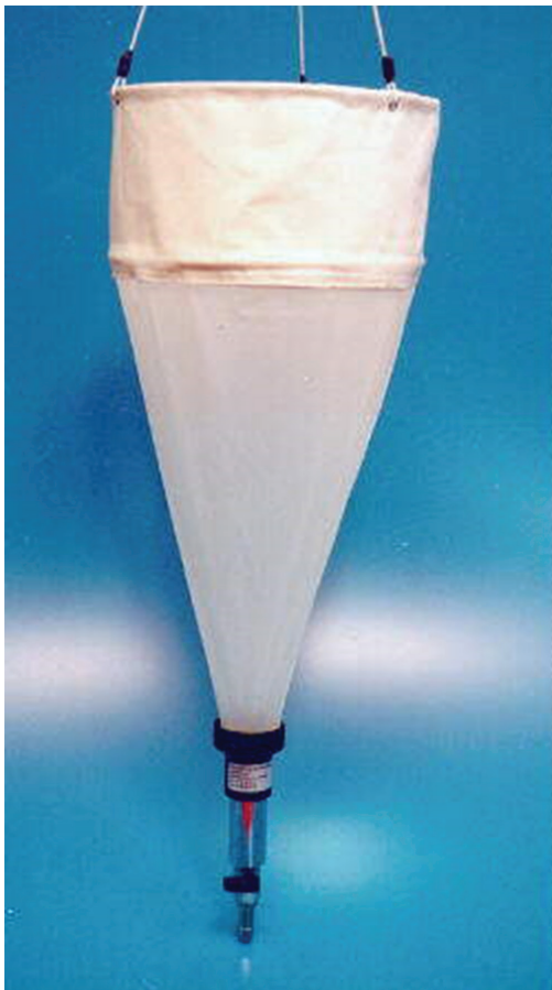
Figure 3. Left: plankton net with a cod end with a stopcock for unloading the sample. Right: plankton net with a cod end, or collection cup, and a weight attached for the descent into the water (model provided to participants in Project RLA/7/014).
