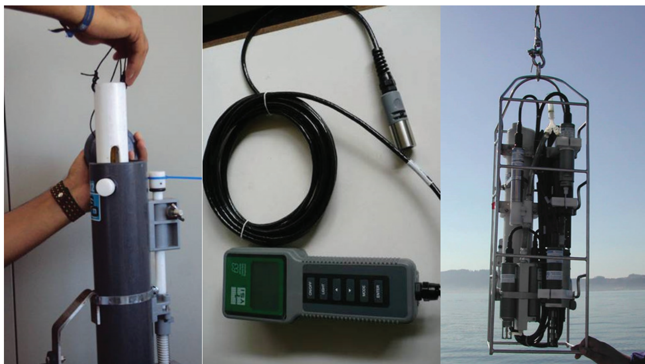
Figure 1. Left: using an immersion thermometer inserted directly into the water-sampling bottle. Centre: YSI multiparameter probe for measuring temperature and salinity. Right: CTD (conductivity, temperature, depth) multiparameter probe attached to the winch of the boat before being cast.
