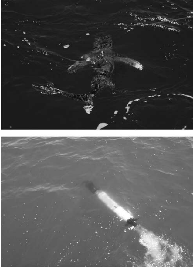
Figure 6.9 Two varieties of autonomous platform used for optical measurements. The rich blue of the oligotrophic waters contrasts with the oceanic white-tip shark, a species being used as a data collection platform by surgically implanted devices. The dark green waters of the coastal environment are a backdrop for the REMUS autonomous vehicle, which has been used for the measurement of the three-dimensional optical structure of the coastal ocean.
