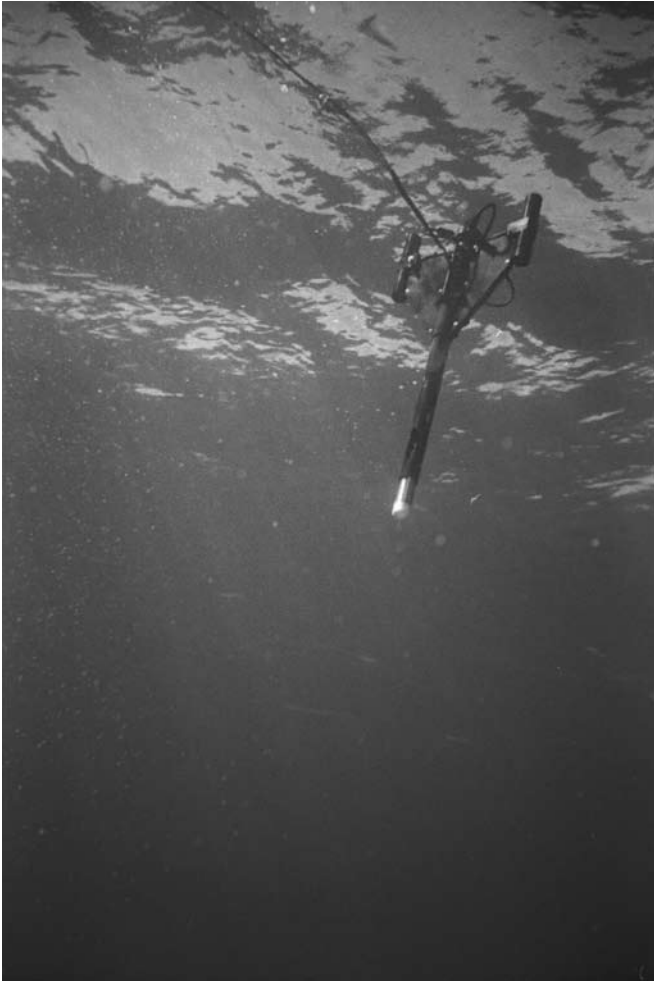
Figure 6.7 Free-fall platform for the measurement of apparent optical properties in the sea.
