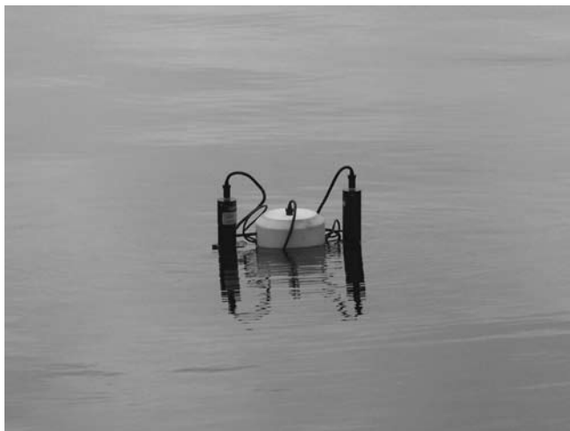
Figure 6.8 Surface buoy platform for the measurement of upwelling irradiance and radiance just below (6–8 cm) the sea surface.
