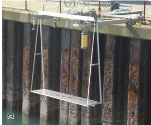
Figures 1 [b], [c]. The same frame and gauges with a metal target (stirrup) suspended beneath them.
