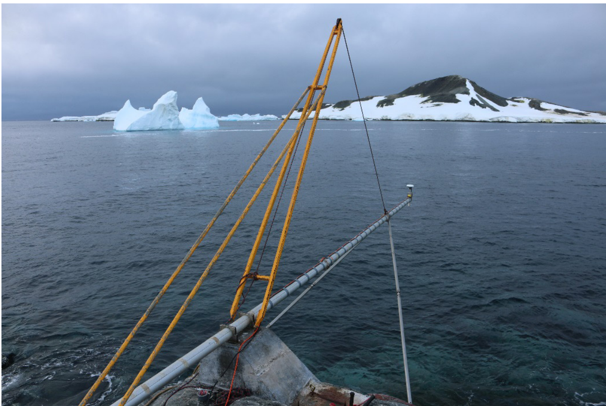
Figure 5 Auxiliary construction (yellow) for assembly and disassembly of the radar gauge arm in GARS O'Higgins.
