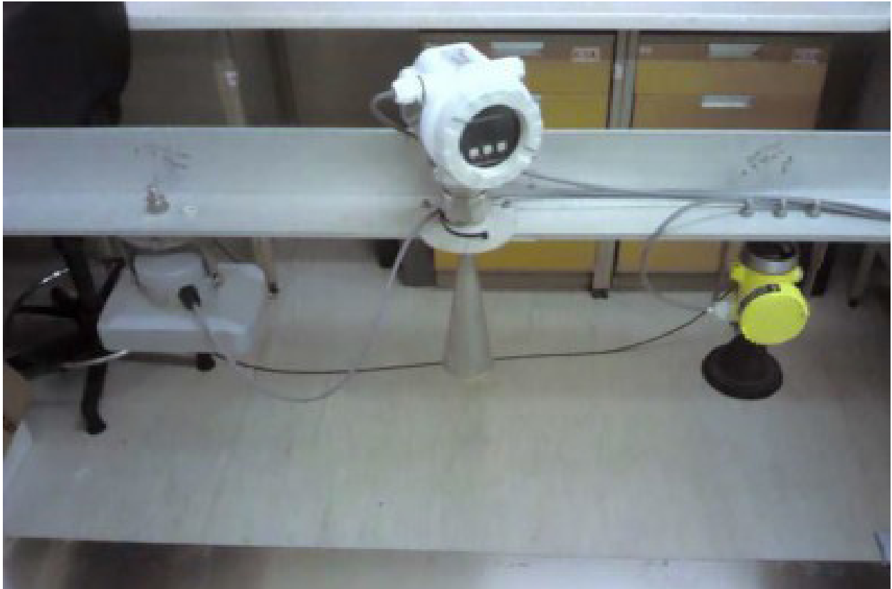
Figure 3. Radar testing in the laboratory showing the same three gauges above the stirrup used at Holyhead. Separate tests were made with a water pool instead of the stirrup.
