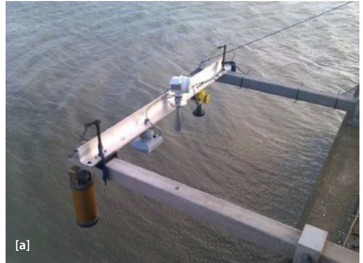
Figure 1 [a]. The test frame at Holyhead holding (left to right) an OTT Kalesto that was not part of the test, an OTT RLS, a Waterlog H-3611 and a VEGAPULS-61. In this photograph the gauges are measuring the sea surface.
