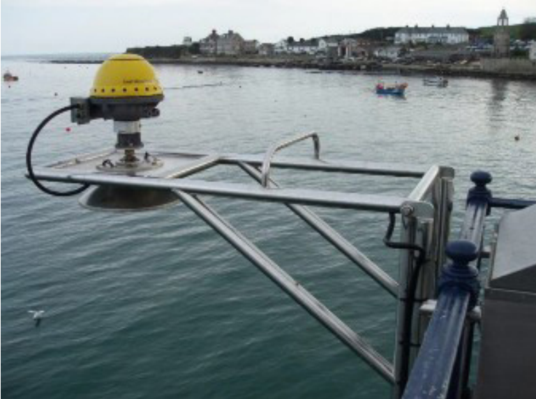
Figure 2. WaveRadar REX on Swanage Pier © New Forest District Council.
