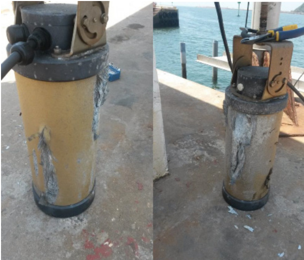
Figure 2. Durban's transducer showing corrosion damage.
