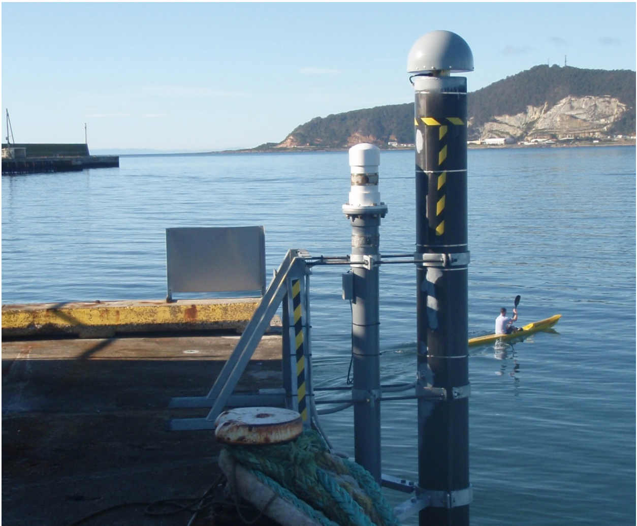
Figure 6.4 An acoustic tide gauge at Burnie in northern Tasmania, Australia, and, to its right, a special pillar with a GNSS antenna on top. Photograph courtesy of Geoscience Australia. From Pugh and Woodworth (2014).
