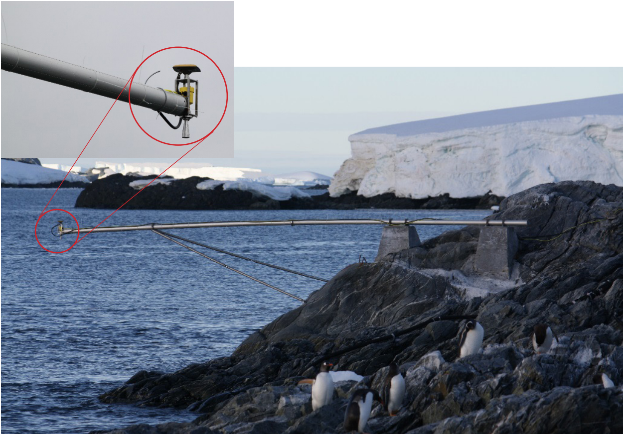
Figure 4 Mount of the radar gauge at the cliff edge in GARS O'Higgins.
