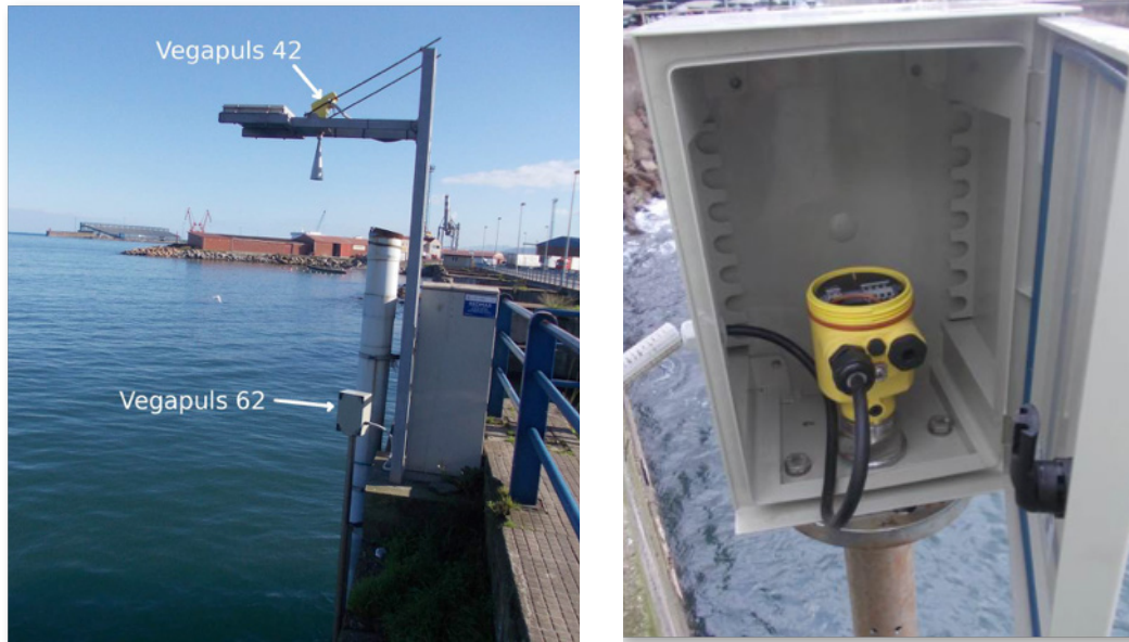
Figure 2. Test station established by SIDMAR technicians at Gijón REDMAR station. Two pulse radar sensors were installed beside the Miros, one measuring inside a stainless steel stilling well (the VegaPuls62, see detail on the right figure) and the other (a VegaPuls42) in the open air, nearby the Miros antenna (left).
