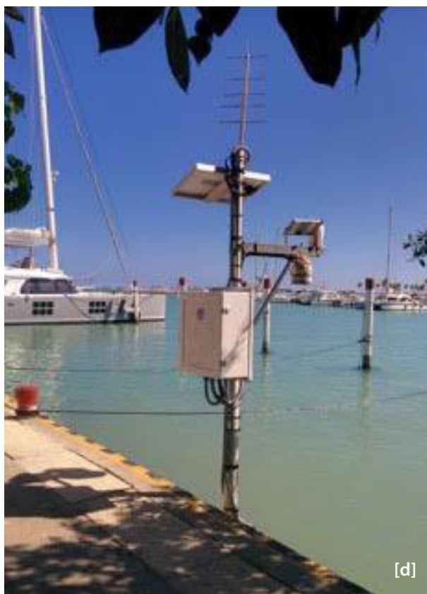
Figure 2 [d]. Punta Cana sea level station operated by the University of Hawaii Sea Level Center (UHSLC) with the National Office for Meteorology in the Dominican Republic (ONAMET). This single radar configuration is similar to that used by UHSLC at this as well as 9 other stations in the Caribbean and Adjacent Regions (Photo Credit: Nikolai Turetsky, UHSLC)
