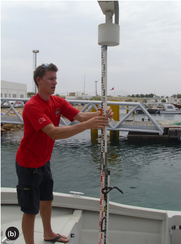
(b) An unusual type of levelling, of an Indonesian radar gauge from a boat in calm conditions (Photograph T. Schöne, GFZ).
