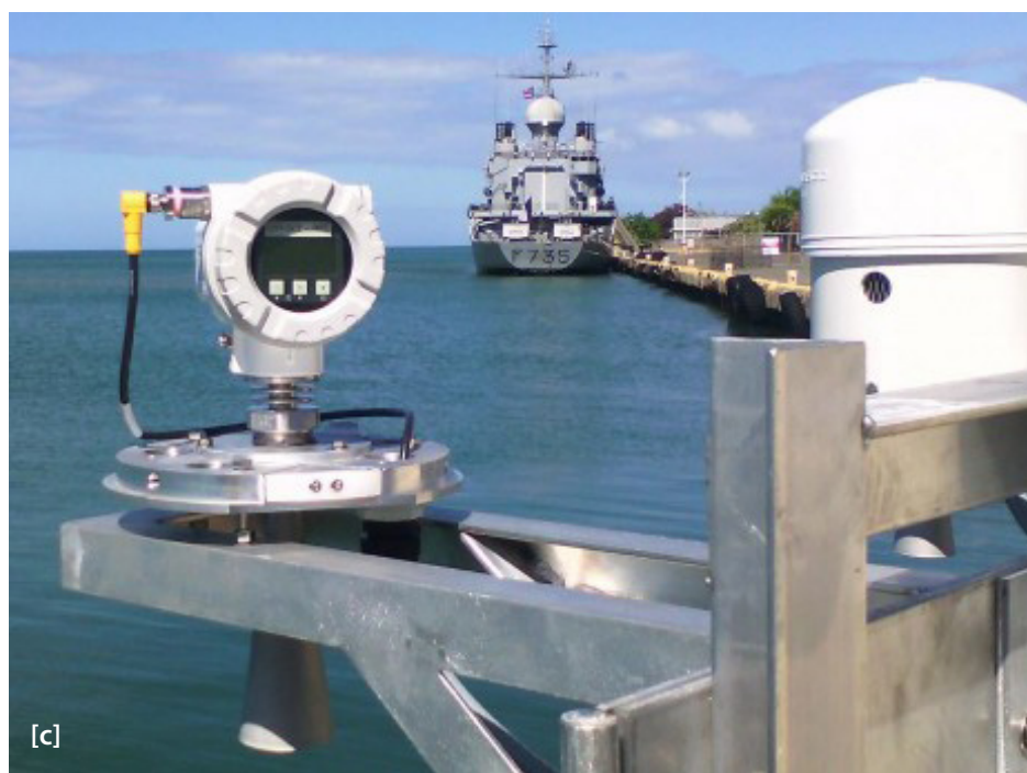
Figure 2 [c]. Double radar sensor configuration in Mayagüez, Puerto Rico (Credit Photo: Jose Cancel, Puerto Rico Seismic Network).
