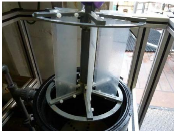
Figure 4.6.2: Silicone rubber sheets mounted in a rack (by courtesy of CEFAS).
