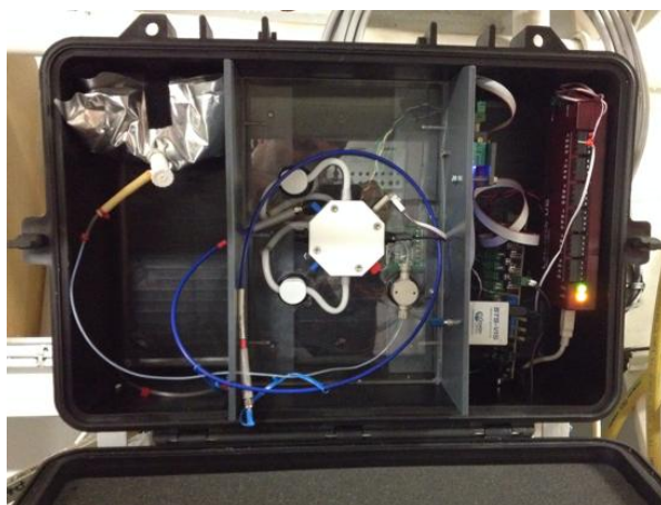
Figure 4.4.8. NIVA spectrophotometric pH-sensor mounted on MS Trollfjord.
