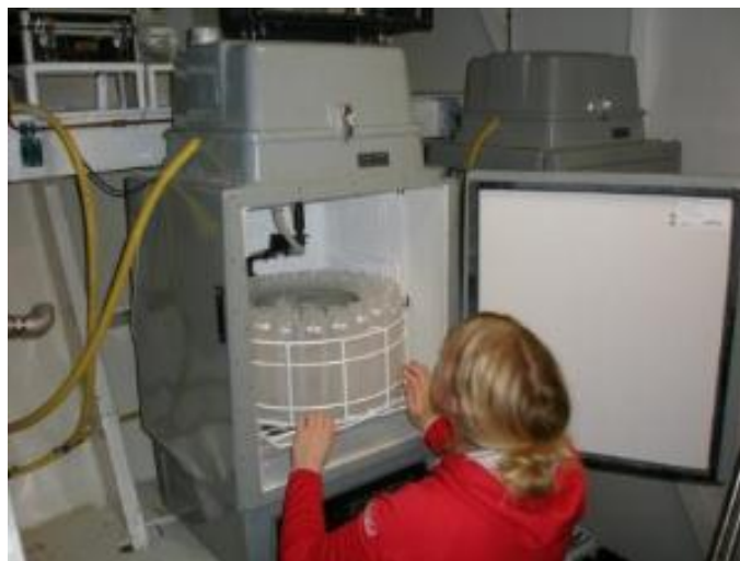
Figure 4.7.1 Automatic water sampling for TransPaper.
