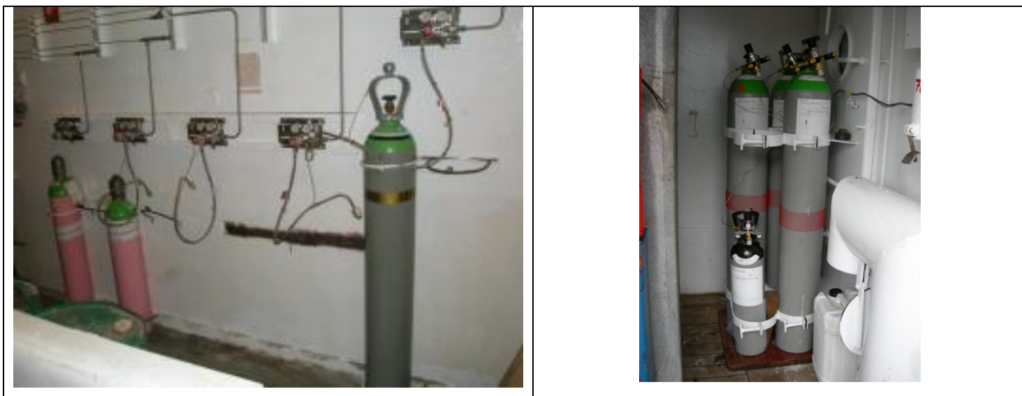
Figure 4.4.3. The General Oceanics CO 2 -system includes analysis of reference gases. Here is the installation on TransPaper (left) and on the NOC reference gas installation on RV Endeavour (right).
