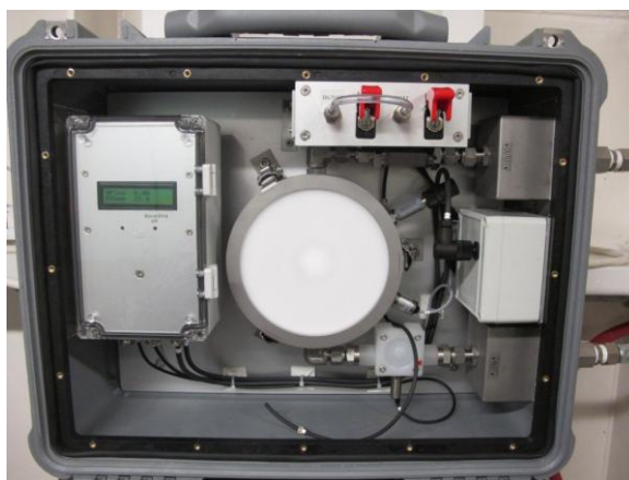
Figure 4.4.6. The NIVA-Franatech membrane based FerryBox pCO 2 system.
