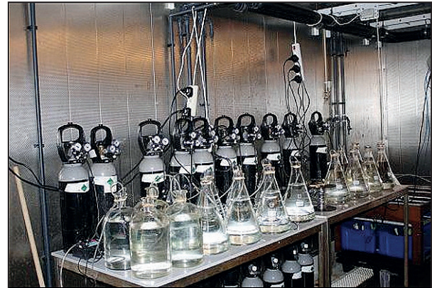
Figure 7.3 Larval cultures at the Sven Lovén ocean acidification facilities (University of Gothenburg). pH is dynamically controlled using pH-computers (Aquamedic) by injection of pure CO 2 in 5 l closed-circuit aquaria allowing an accuracy of 0.04 pH units (photo credit: S. Dupont).
