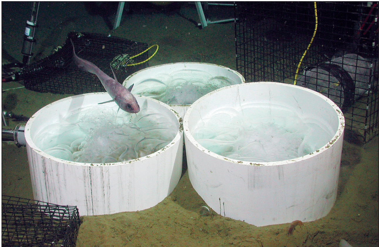
Figure 8.2 Photograph of manipulative deep-sea experiment to evaluate the response of deep-sea organisms to low pH / high p(CO 2 ). Liquid CO 2 (~60 l) was released into PVC tubes (~45 cm diameter) placed on the seafloor at 3600 m depth off central California. The liquid CO 2 dissolved into seawater, producing a high CO 2 , low pH plume that drifted over the seabed and organisms in the sediment or held in cages at different distances from the CO 2 pools (photo credit: J.P. Barry).
