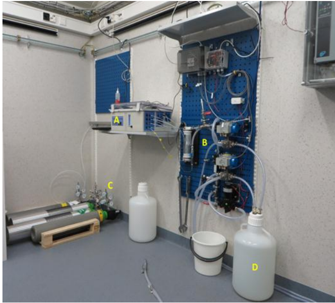
Figure 3.3.3. SuperCO 2 measuring system at Utö Atmospheric and Marine research station. (A) instrument, (B) equilibrator and valves, (C) calibration gases and (D) container for cleaning agent.
