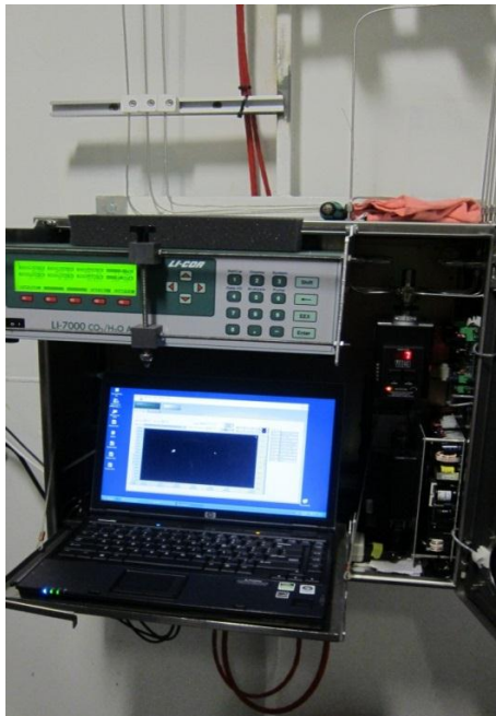
Figure 3.3.1. (left) Dry box with LICOR and computer visible. (right) Wet box with EQU, main filter (blue cap) and temperature measurement (yellow).
