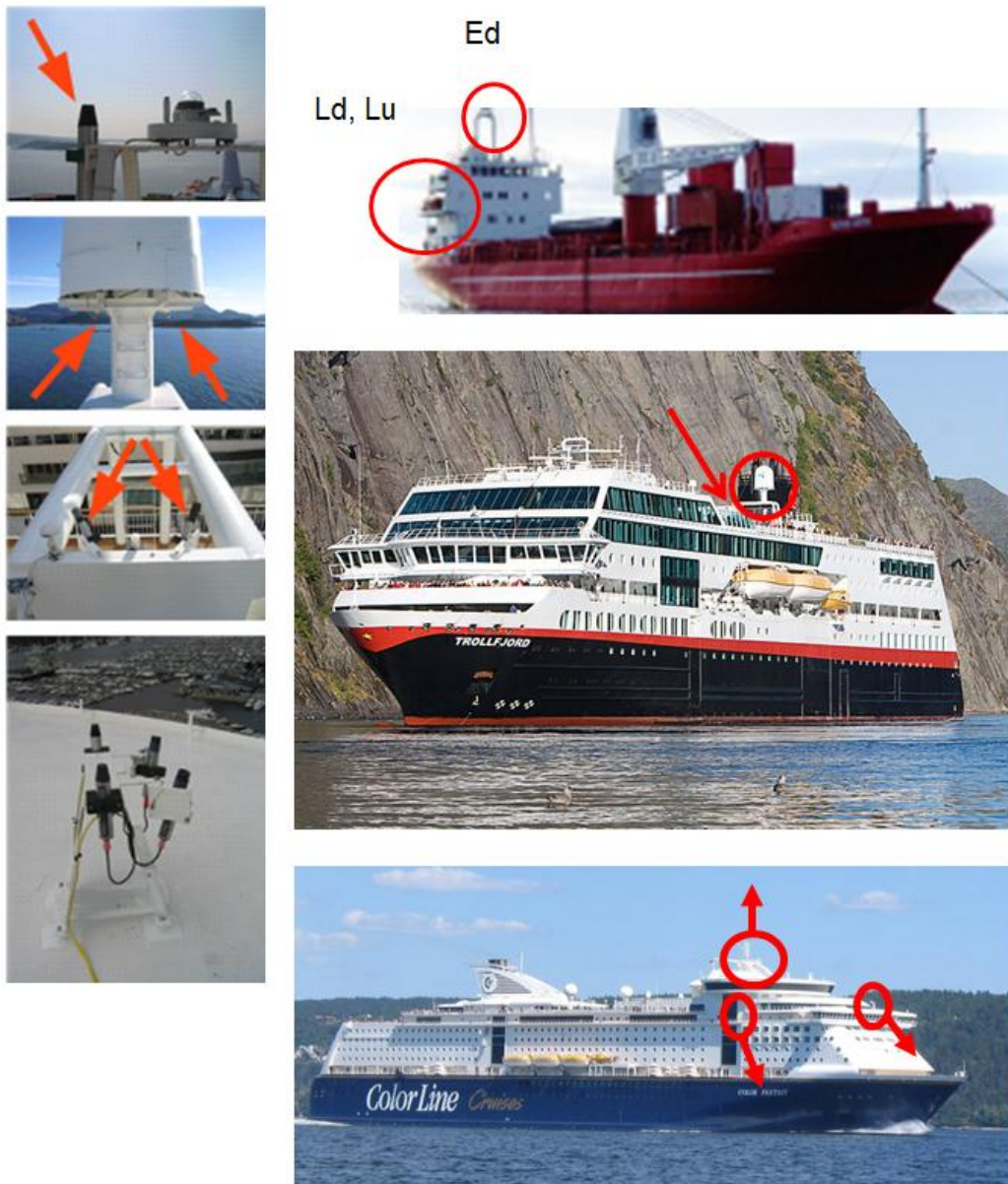
Figure 3.2.11. Left, top to bottom: (1) irradiance sensor on top of mast installed on ship (C), (2) downward looking radiance sensors below antenna dome on ship (B), upward looking radiance sensors on ship (B) and upward looking sensors on ship (C). Right, ship installations. Top to bottom: (A) 1 pair of radiance sensors is placed on the back and irradiance sensor in the mast. (B) 2 pairs of radiance sensors, one looking forward and the other backward. The downward looking sensors are placed below the antenna dome. (C) 2 pairs of radiance sensors, one looking on starboard and the other on port side. The downward looking sensors are placed just below the bridge all other instruments being installed on the monkey deck.
