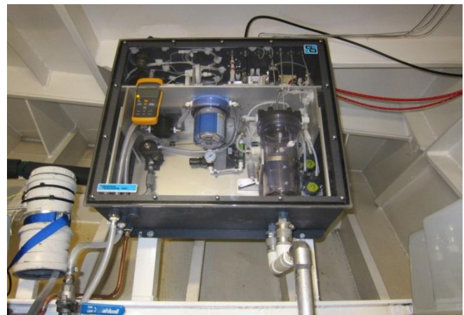
Figure 3.3.1. (left) Dry box with LICOR and computer visible. (right) Wet box with EQU, main filter (blue cap) and temperature measurement (yellow).
