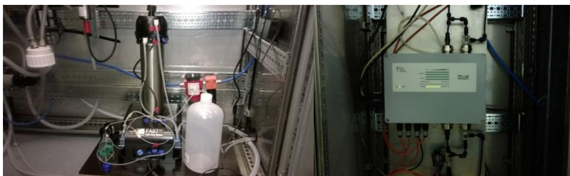
Figure 3.2.5. Commercial FRR fluorometers: FastOcean (left) and FFL-40 (right)
