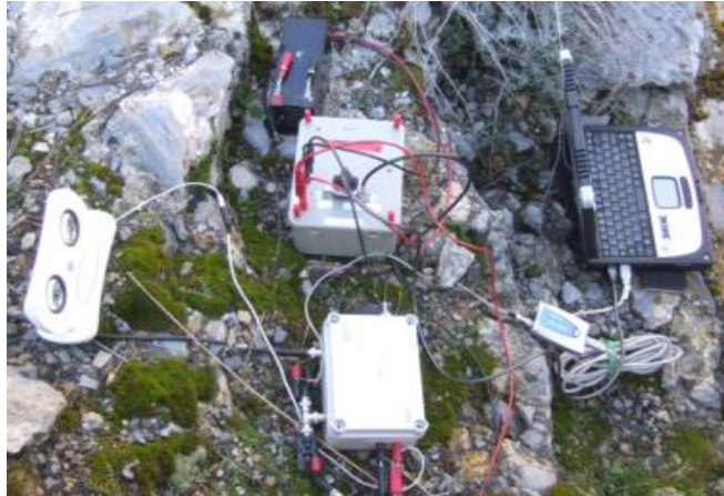
Figure 6. A simple radio setup used by the Nato Undersea Research Center, Italy, to monitor the HF-radio band for identifying the most suitable frequency and site from the standpoint of background noise.
