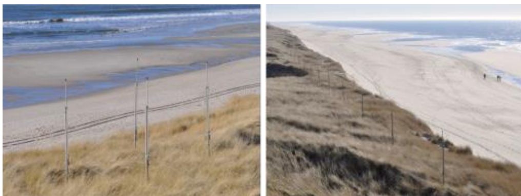
Figure 2. The photos show a phased array setup of a Wera system on the island of Sylt on the German coast of the North Sea. The left hand side shows the transmitter antenna array (Tx) and the right hand side the receive array (Rx). The system is one of the three HF-radars installed within the framework of the COSYNA Project to help monitor the German Bight.
