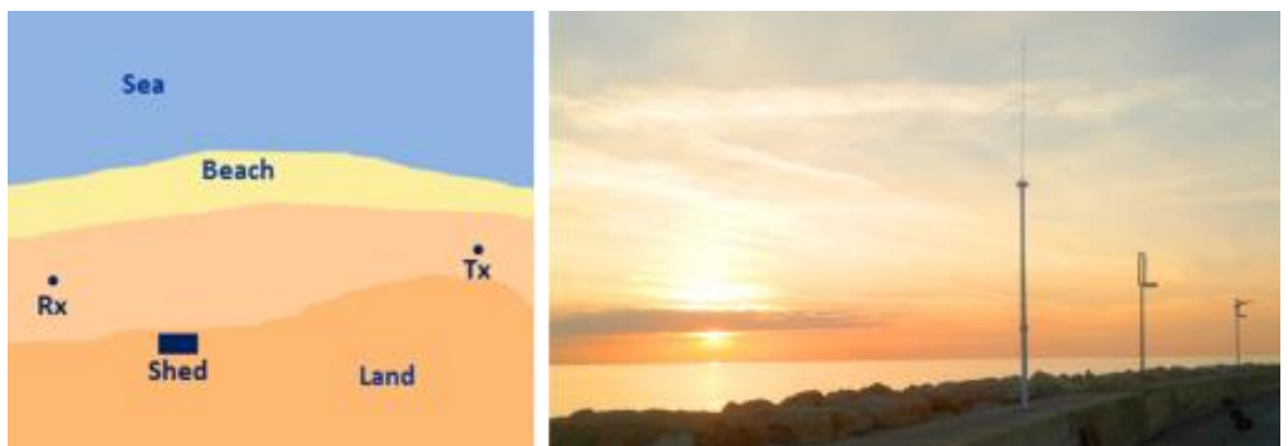
Figure 3. The left panel illustrates a typical setup of a standard/long range direction-finding HF-radar system. The right panel shows a SeaSonde direction-finding system installed at Marina Di Ragusa in Sicily, Italy. This system is one of the four HF-radars that were set up within the CALYPSO Project to monitor sea-surface currents in the Malta-Sicily Channel.
