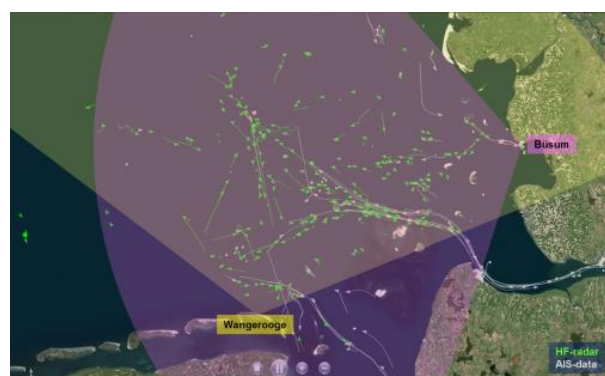
Figure 5. Map of ship detects in the German Bight resulting from the fusion of HF-radars at Wangerooze and Büsum, covering the German Bight of the southern North Sea. The ship detects are plotted in green and the corresponding positions of the Automatic Identification System (AIS) are depicted in grey.
