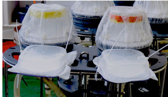
Fig. 4: Dipped blank filter sets sandwiched between 1 \mu\text{m} polyester mesh, and deployed in perforated plastic containers that are attached to the pump with cable ties.
