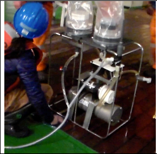
Fig. 5. On-deck evacuation of seawater from filter holder headspace using vacuum lines to an aspirator pump on deck.
