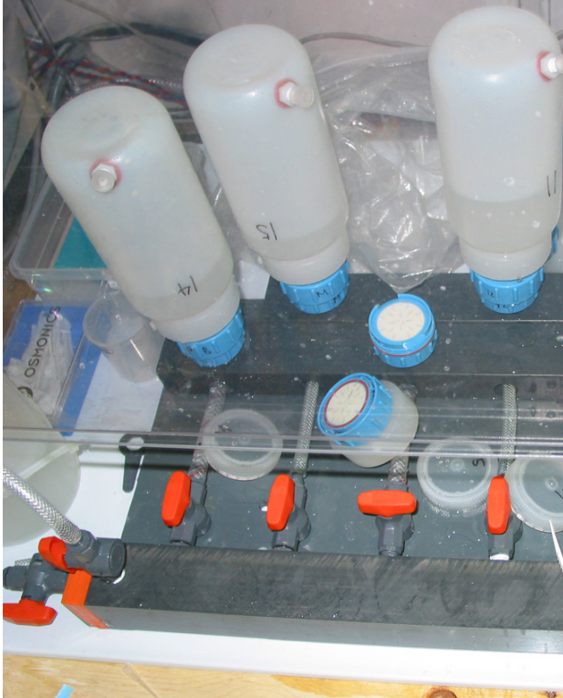
Figure 3. An example of a 1 L offline filtration method as used routinely on CLIVAR A16N, A16S, VERTIGO, and GEOTRACES IC expeditions. Pre-cleaned 1L LDPE bottles are modified with closing air vents at bottom. Sample is quickly transferred from the GO-FLO into the 1 L LDPE bottle which is then capped conventionally. Once returned to a Laminar Flow bench environment, the top is substituted for a tapered adaptor which has a mated 47 mm MFS filter holder with preloaded 0.45 \mu\text{m} Supor filter. The upstream orifice of the filter holder has been drilled out to twice standard diameter to minimize air-lock effects. Once samples are filtered under 25 to 40 mm Hg vacuum, they are transferred directly to sample bottles for further processing. Primary sample bottles and filter holders are reused after TM-clean DI water rinsing. More information available from J. Bishop ( jbishop@berkeley.edu ) or Todd Wood ( tjwood@lbl.gov ).
