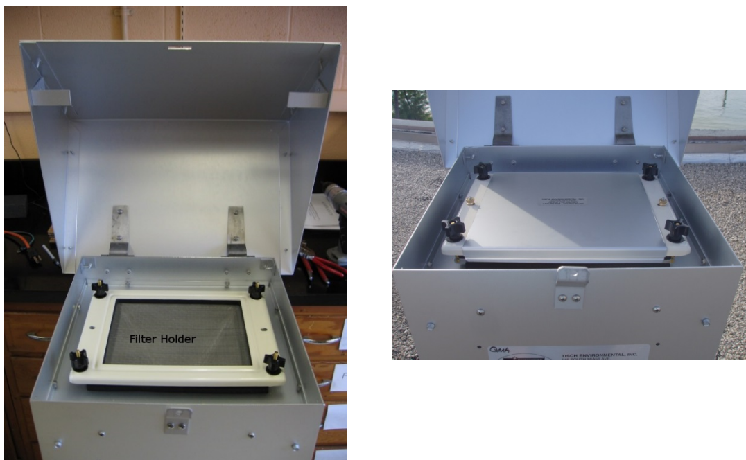
Figure 2. Large format (25.4 cm x 20.3 cm) filter holder and filter holder with the cover.
