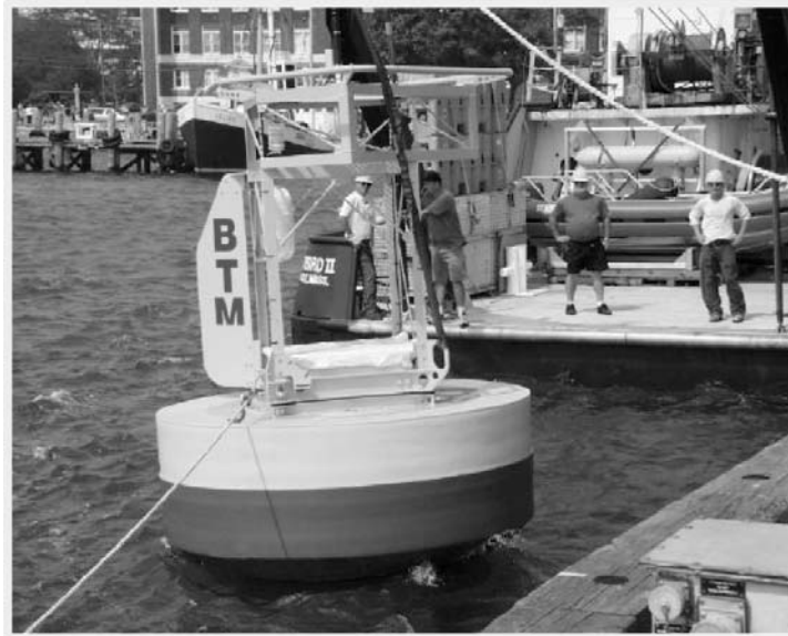
Fig. 3.8: Photograph of the newly designed and recently deployed interdisciplinary BTM surface buoy ( www.opl.ucsb.edu ).
