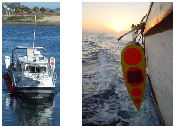
Figure 1.10. Pole-mounted transducers. Hydraulically retractable poles (left) are used to mount multibeam (starboard) and multifrequency split-beam transducers (port) on a small craft. A manually retractable pole is used aboard a fishing boat and other platforms of opportunity (right).
