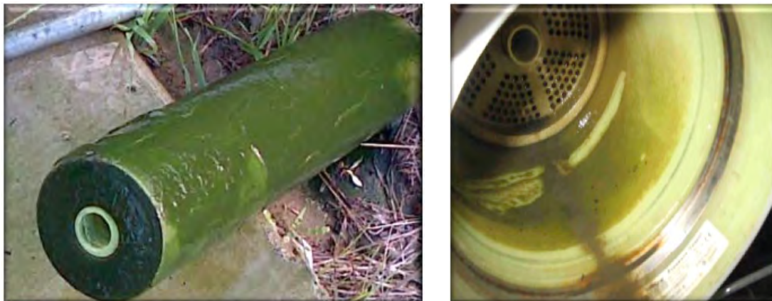
Figure 1. Severe fouling due to algal bloom. Algal fouling on a cartridge filter (L), remnants of algal fouling left inside a pressure vessel after removing the lead element (R). Note: Elements are from a brackish water reverse osmosis system, fouling may appear as different colors in a SWRO system.
