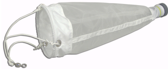
Figure 3.6 A plankton net, used to collect large amounts of biomass. Note that these types of samples are not quantitative.
