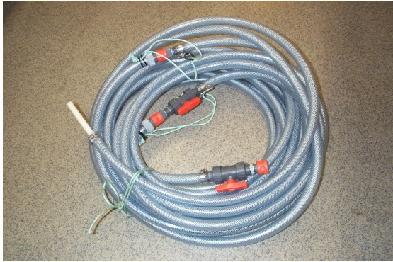
Figure 3.5. A hose used for phytoplankton sampling. The valves are open when lowering the hose into the water. The top valve is closed before lifting the tube out of the water. Photo: B. Karlson.
