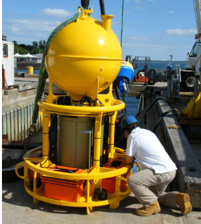
Figure 3.20. The Environmental Sample Processor (green canister), an autonomous “laboratory in a can” that can detect and enumerate HAB species and measure toxins. Photo: Woods Hole Oceanographic Institution.
