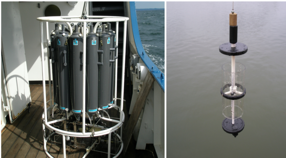
Figure 3.4. Water sampling devices. Left: Individual Niskin-type bottles mounted in a rosette for sampling at multiple depths on a single cast; right: a water sampling device of the Ruttner type. Photo: B. Karlson.
