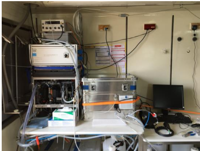
Figure 3.3.14: Sensor set-up during both cruises. From left to right: FerryBox connected to water inlet, HyAbS inside Zarges-box, Oscar G-2 inside black pressure housing
