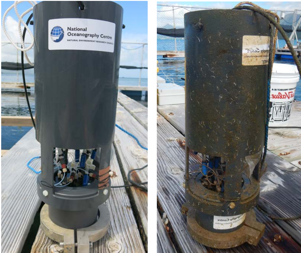
Figure 22. Photographs of the NOC-PO4 prior to and following the one month HIMB field trial.
