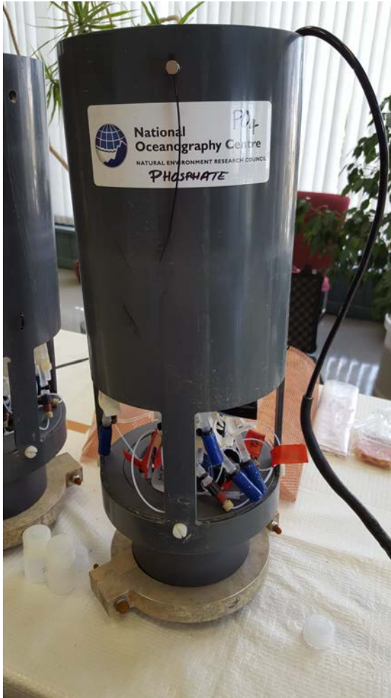
Figure 12. Photographs of the NOC-PO4 prior to and following a 32 day field test in the Maumee River.
