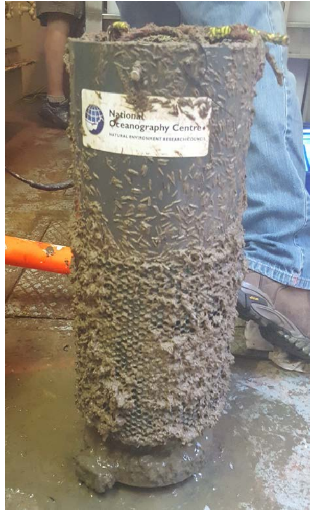
Figure 12. Photographs of the NOC-PO4 prior to and following a 32 day field test in the Maumee River.
