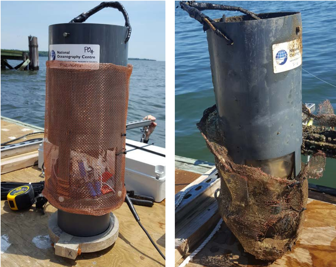
Figure 17. Photographs of the NOC-PO4 instrument prior to and following the CBL field trial.
