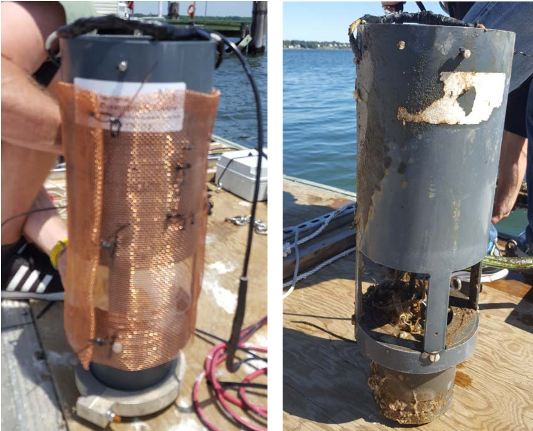
Figure 17. Photographs of the NOC-NO23 instrument prior to and following the CBL field trial.
