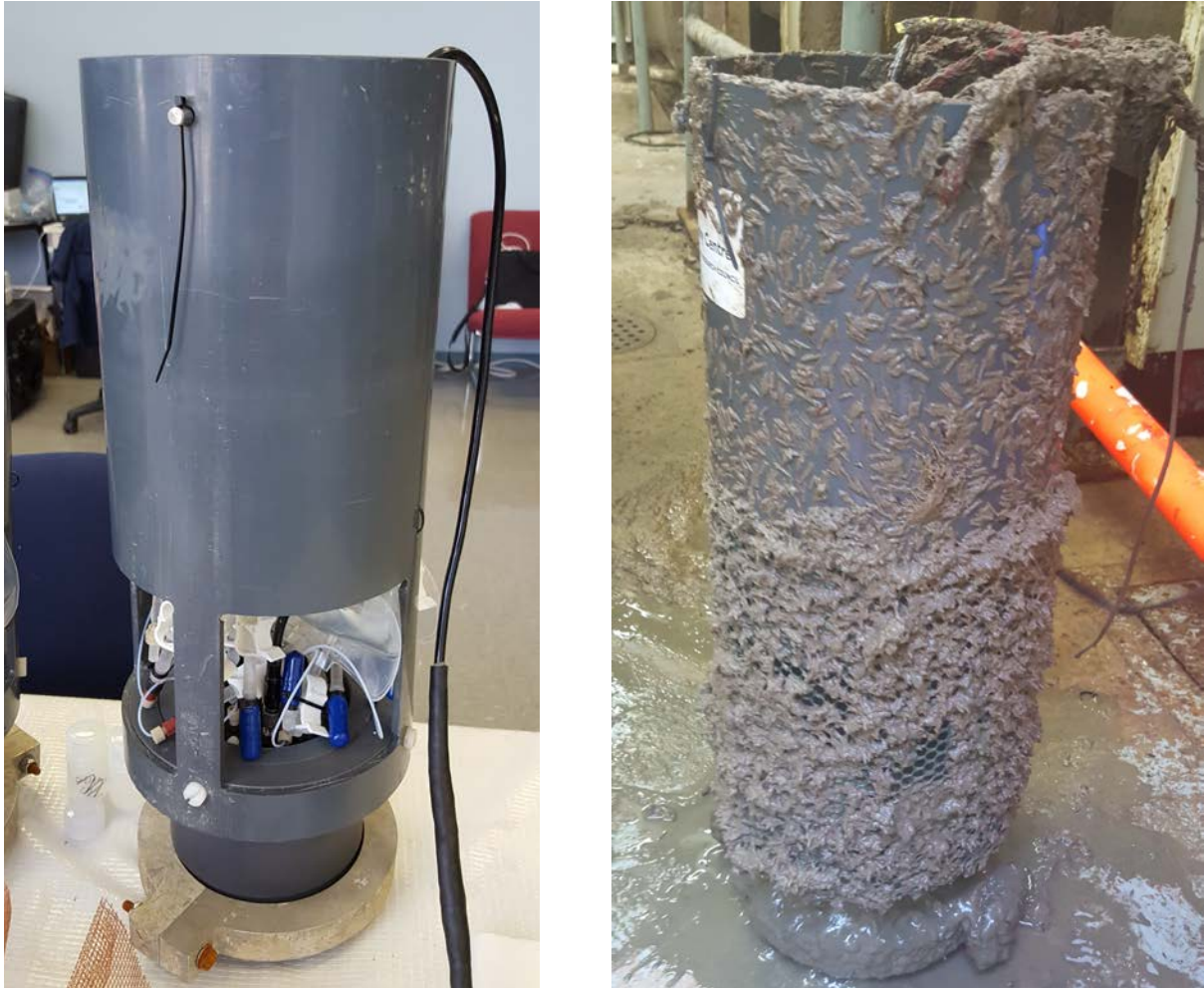
Figure 12. Photographs of the NOC-NO23 prior to and following a 32 day field test in the Maumee River.
