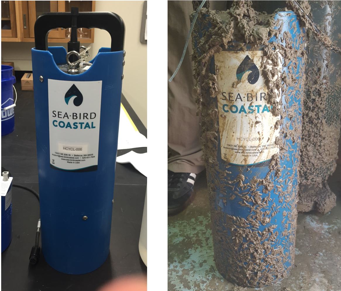
Figure 12. Photographs of the HydroCycle-PO4 prior to and following a 32 day field test in the Maumee River.
