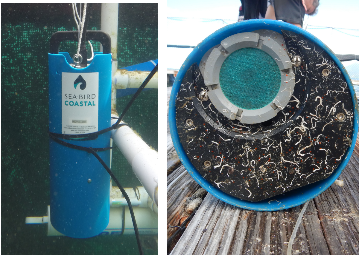
Figure2. Photographs of the HydroCycle-PO4 prior to and following the one month HIMB field trial.
