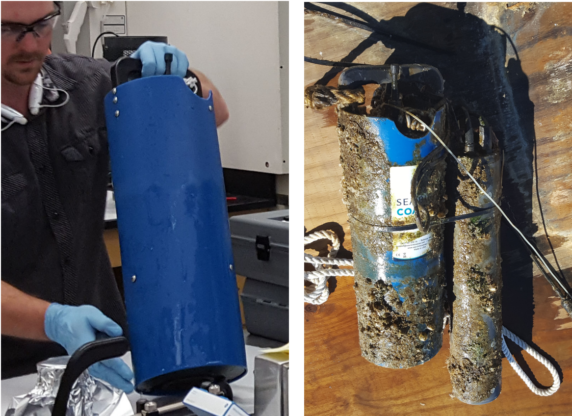
Figure 17. Photographs of the HydroCycle-PO4 instrument prior to and following the CBL field trial.
