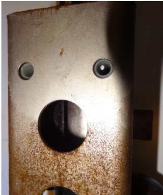
Photo 2. SBS HydroCAT prior to and following 15 week deployment under ice for the MTU field test.
