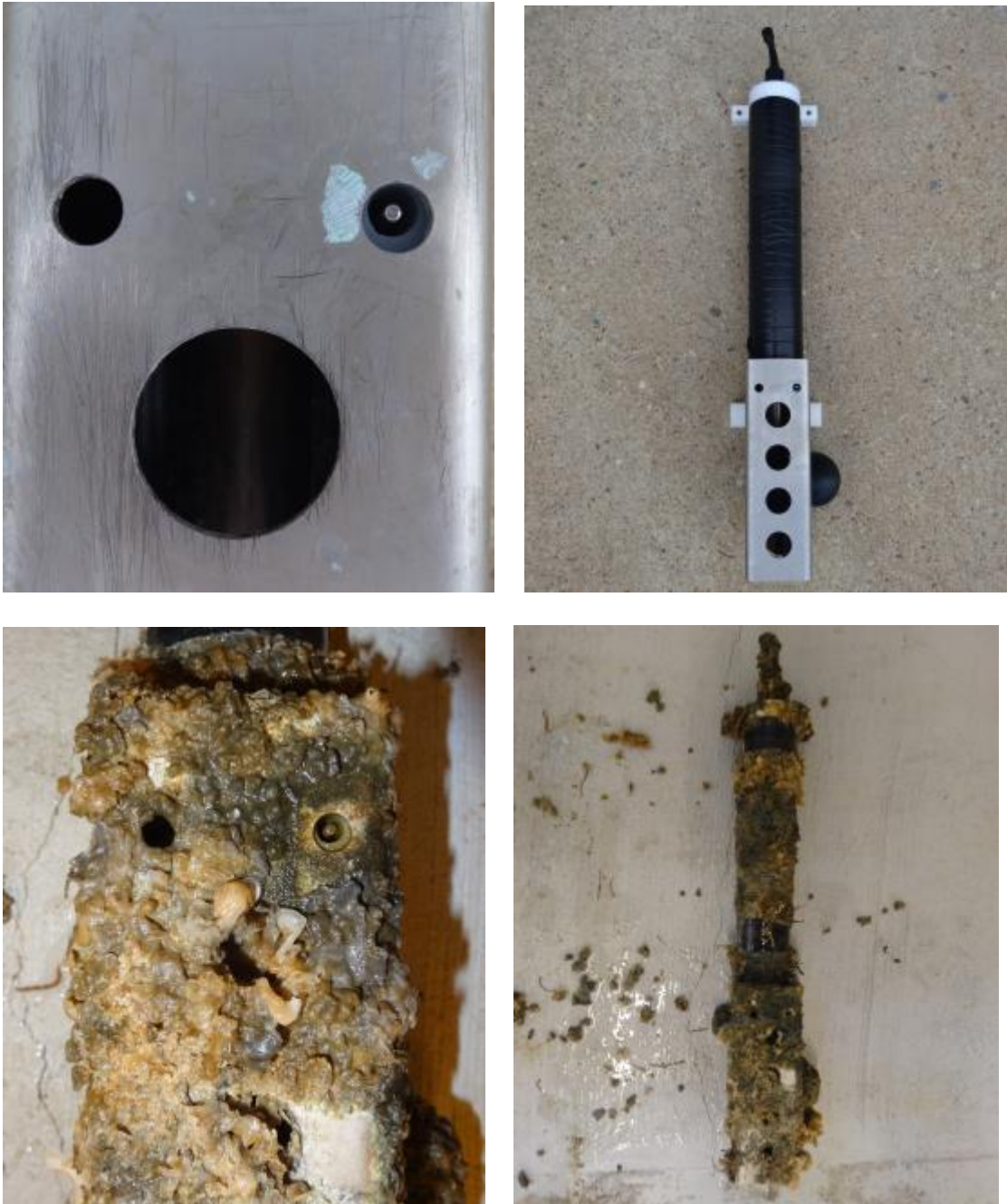
Photo 4. The SBS instrument before and following the 12 week CBL field trial.
