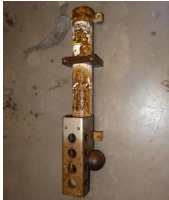
Photo 2. SBS HydroCAT prior to and following 15 week deployment under ice for the MTU field test.
