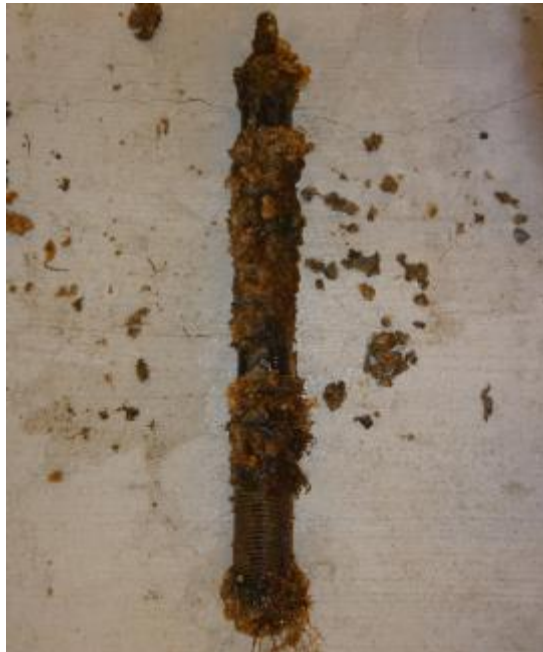
Photo 4. The Troll 9000 instrument and following the 12 week CBL field trial.
