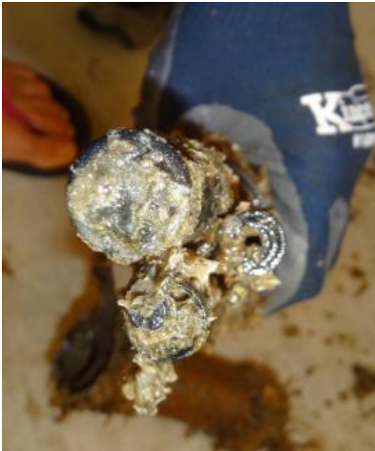
Photo 4. The Troll 9000 instrument and following the 12 week CBL field trial.
