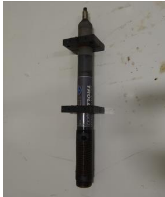
Photo 2. Troll 9000 prior to and following 15 week deployment under ice for the MTU field test.
