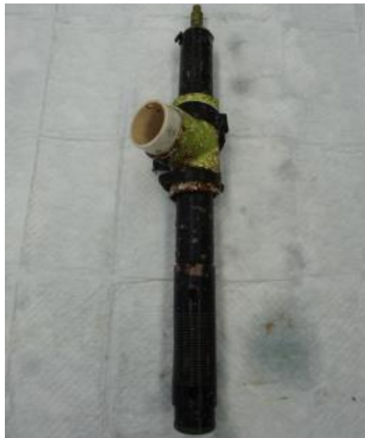
Photo 6. The Troll 9000 prior to and following the 18 week HIMB field trial.
