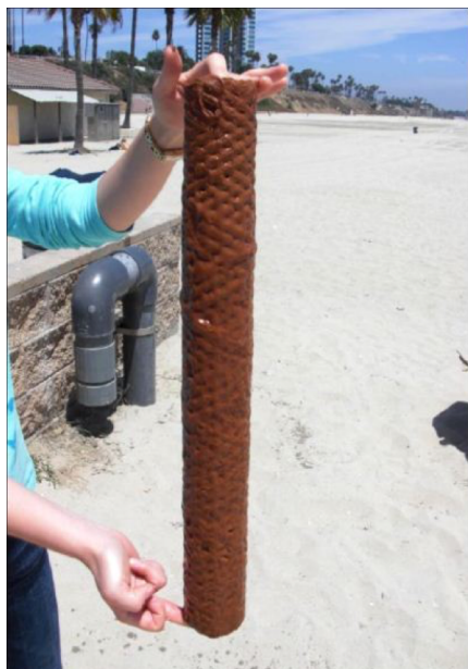
Figure 9.31. Heavily fouled cartridge filter during severe algal bloom event from the Pacific Ocean. Photo: Voutchkov (2013).
