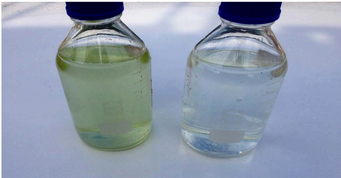
Figure 11.5.9. Samples of feedwater (left) and DAF-treated water (right) from the challenge test at the Fujairah I pilot plant using cultured algae.
