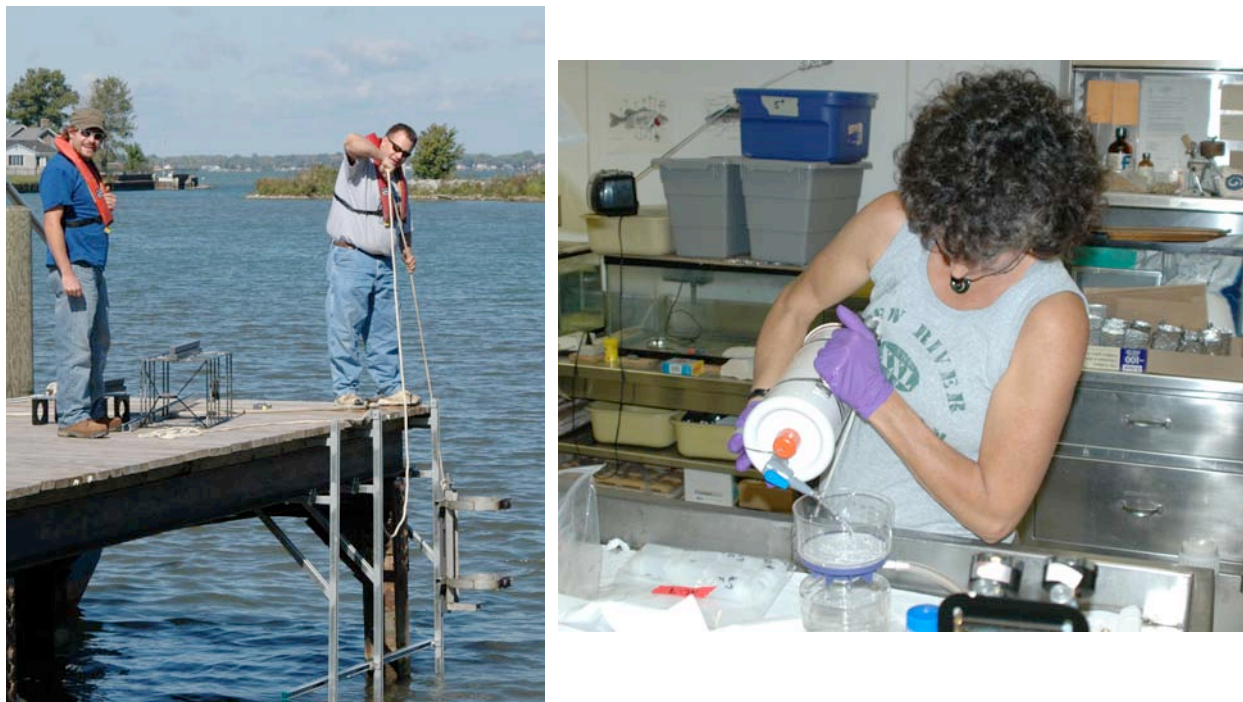
Figure 6. The Michigan field test site was located at the mouth of the Clinton River in Mt. Clemens, MI. The test instrument was deployed on a mooring frame attached to the end of a fixed pier. Collection of reference samples occurred at the same depth and less than 1m apart from the sample inlet. Samples were immediately filtered and frozen in the adjacent laboratory.
