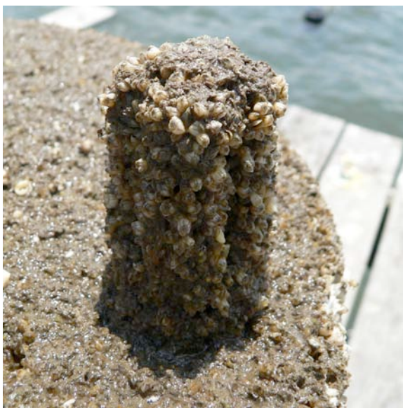
YSI 9600 sample inlet after the deployment
