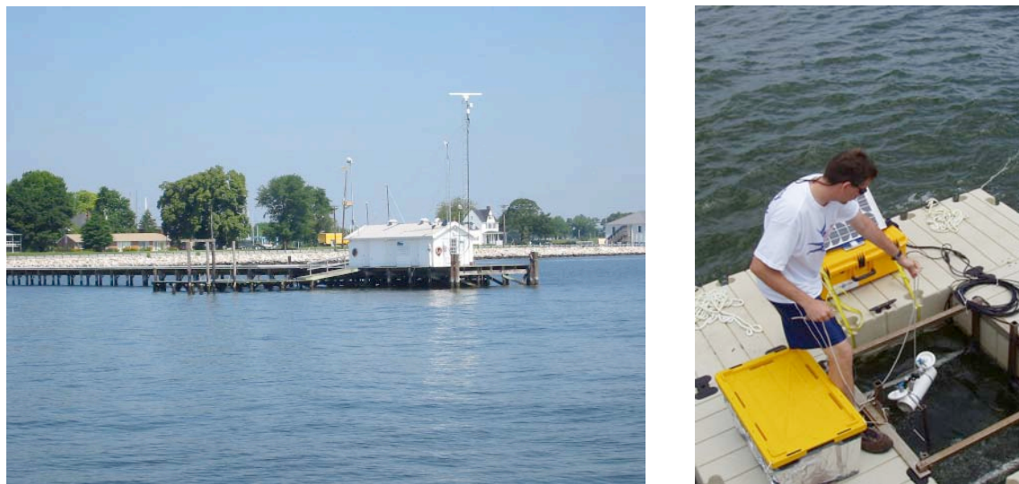
Figure 1. Coastal environment and field test site for the Chesapeake Biological Lab. The test instrument was deployed on a mooring frame constructed within an Easy Dock platform. Collection of reference samples occurred within the middle opening of the platform less than 1m apart from the instruments sample intake.
